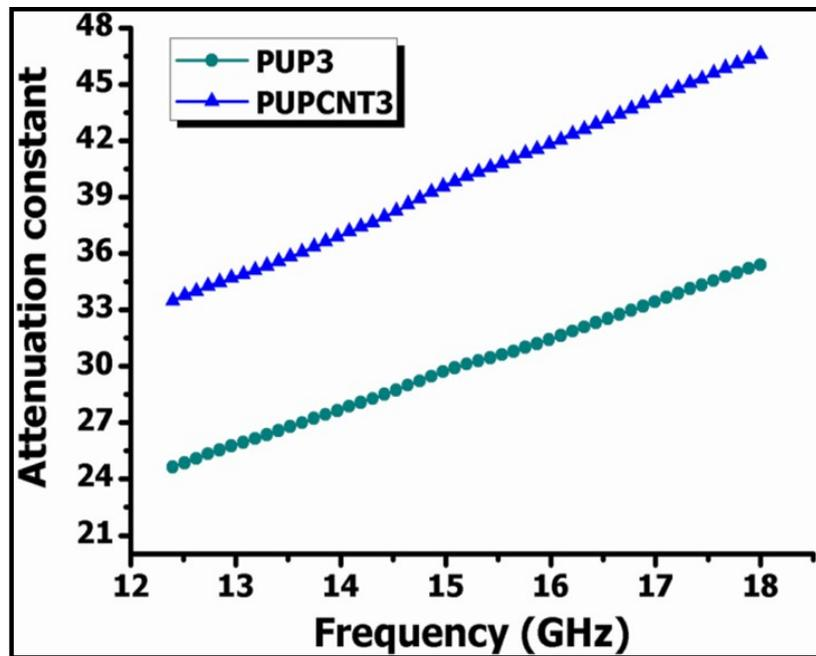
**Fig 2** Attenuation constant of PUP3 and PUPCNT3 composites
