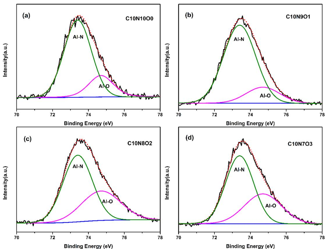
Fig. S1 XPS spectra of Al 2p for samples C10N10O0 (a), C10N9O1 (b), C10N8O2 (c), and C10N7O3 (d) after 10s Ar gas purge, with the experimental spectra depicted with dots and the simulated one with solid lines. All spectra were calibrated with C 1s peak.
