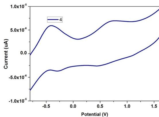
**Figure S4a.** Cyclic voltammograms of fluorescent amidophanes **1**, **2**, **3** and **4** in DCM at room temperature (scan rate at 100 mV s<sup>-1</sup>) and 0.1 M TBAP as a supporting electrolyte in dry DCM.
