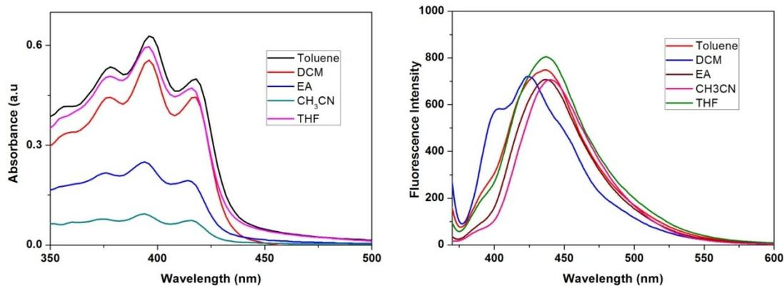
**Figure S1.** The solvatochromism of the fluorescent amidophane **2** of absorption and emission spectrum.
