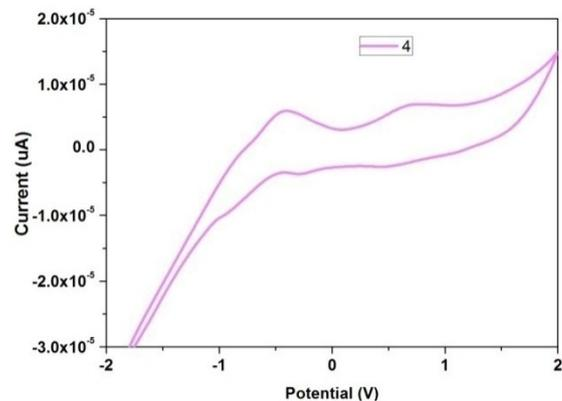
**Figure S4.** Cyclic voltammograms of fluorescent amidophanes **2**, **3** and **4** in DCM at room temperature (scan rate at  $100 \text{ mV s}^{-1}$ ) and 0.1 M TBAP as a supporting electrolyte in dry DCM.
