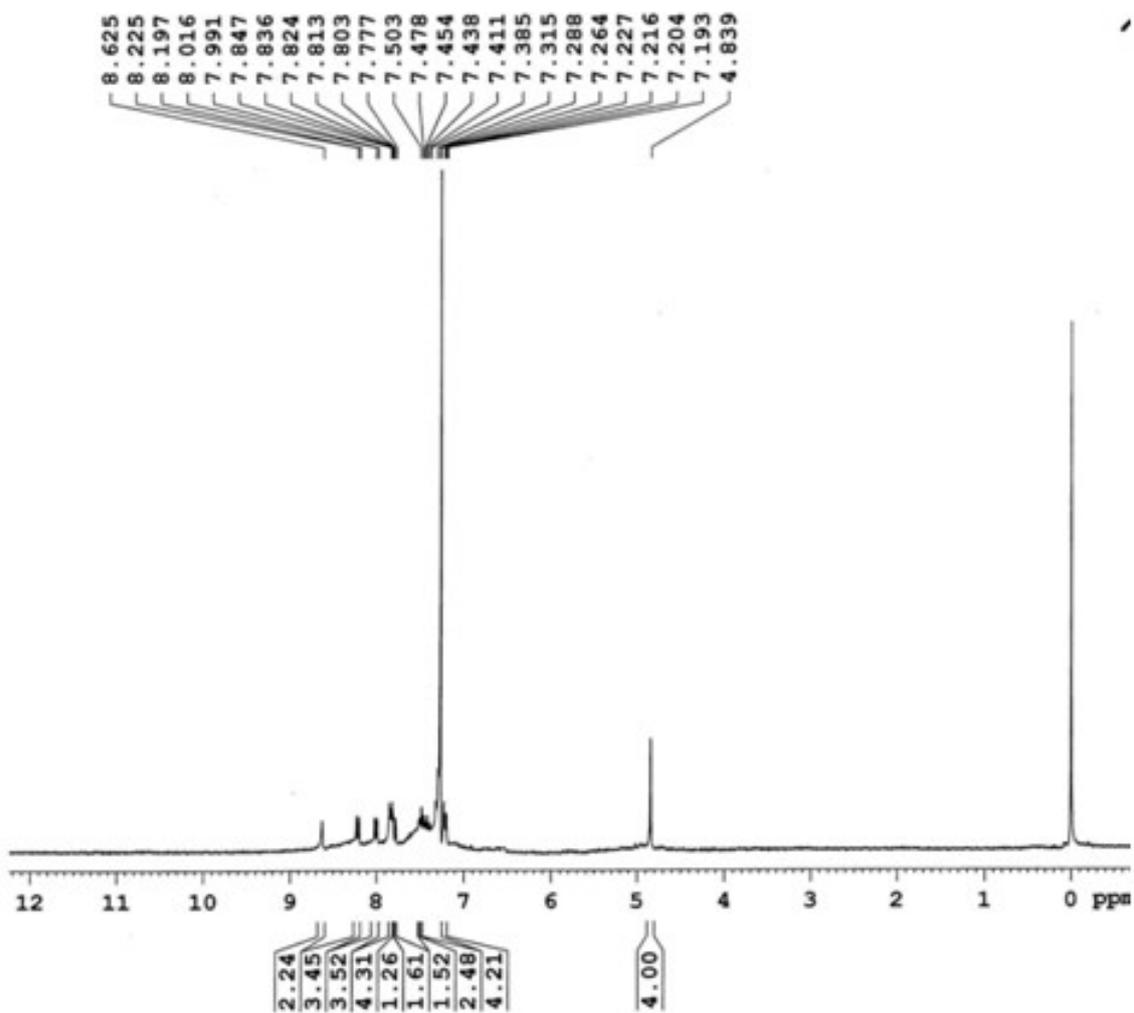
$^1\text{H}$  ( $\text{CDCl}_3$ ) NMR (300 MHz) spectrum of Compound 1
