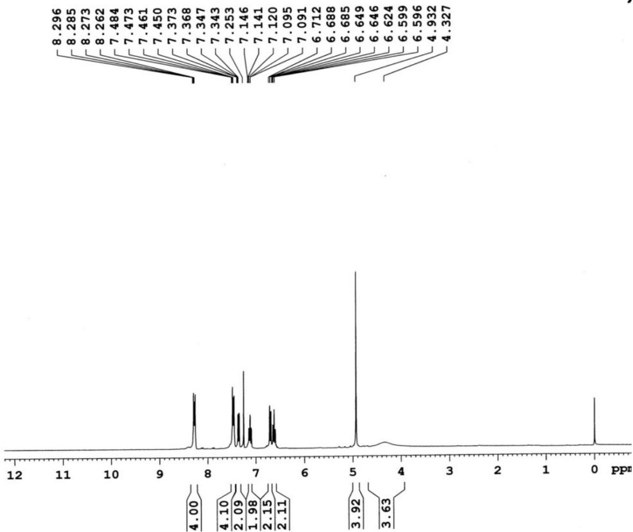
$^1\text{H}$  ( $\text{CDCl}_3$ ) NMR (300 MHz) spectrum of Compound 7
