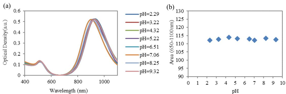
Figure S1 a) UV- Vis spectra of original Au NRs in different pH and b) corresponding surface area of Au NRs at the range of 650-1100 nm. Variation of pH in the range of 2.29 to 9.32 did not induce any morphology changes on NRs, as there is not significant shift of longitudinal surface plasmon supported by constant surface area at the range of 650-1100 nm at different pH.
