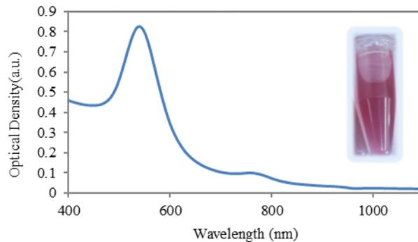
Figure S3 UV- Vis spectrum of Au NRs in presence of 24 mM NaOH. The original growth solution was colorless, but after injection of NaOH, the color of solution turned to reddish along with appearance of a plasmon peak at around 530 nm that is an indication of gold nanoparticles formation.
