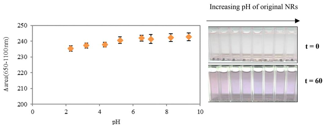
Figure S2 Glutathione-induced overgrowth on Au NRs solution having different initial pH. The concentration of glutathione was 5  $\mu$ M for all cases.
