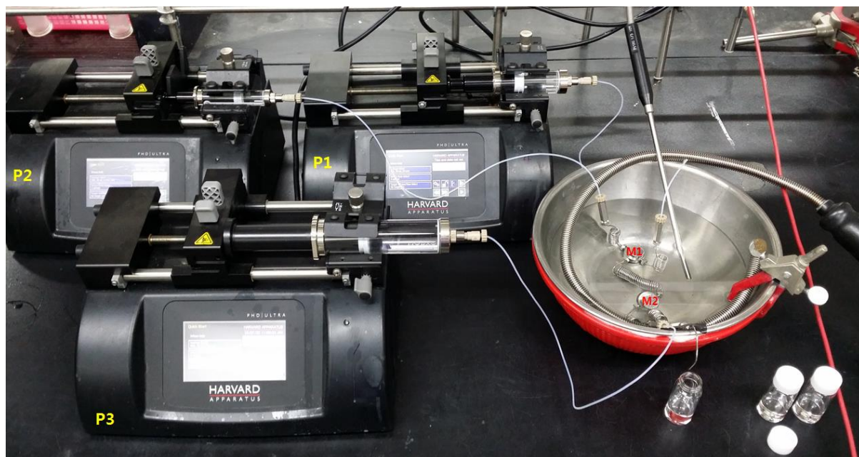
Figure 2. Flow chemistry reaction set-up employed in this study.
