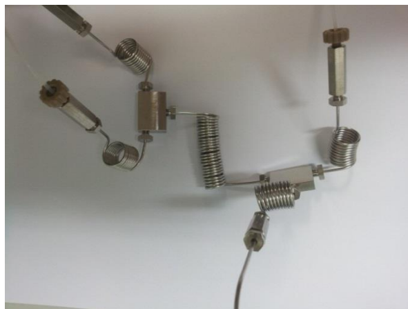
Figure 3. Pre-cooling coil employed in this study.
