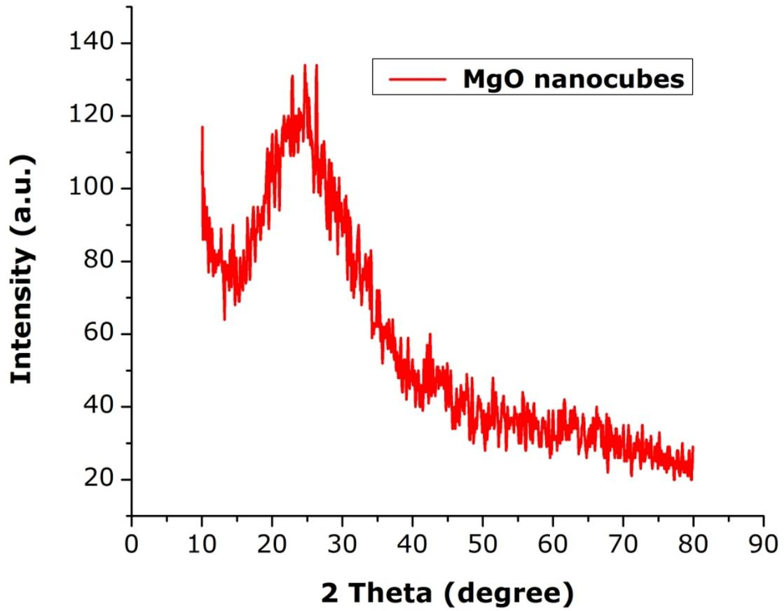
Supplementary Figure S1:- XRD pattern of pure MgO nanocube arrays prepared via hydrothermal method.
