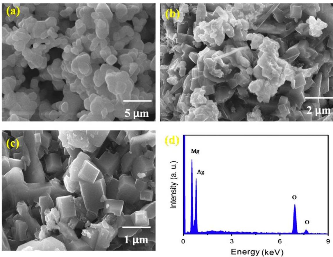
Supplementary Figure S4:- Scanning electron microscopy (SEM) images and Energy dispersive spectrum (EDS) pattern of pure MgO nanocube prepared via hydrothermal method.
