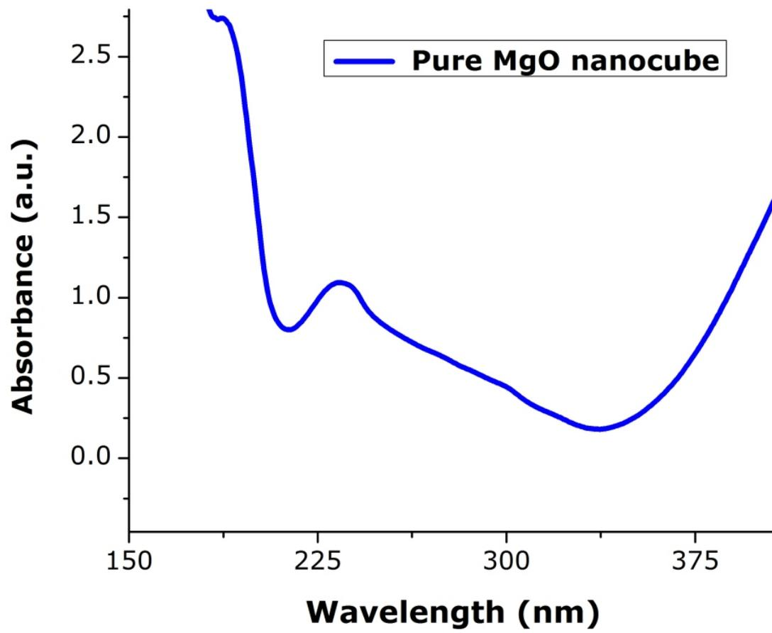
Supplementary Figure S2:- Optical absorption images of pure MgO nanocube prepared via hydrothermal method.
