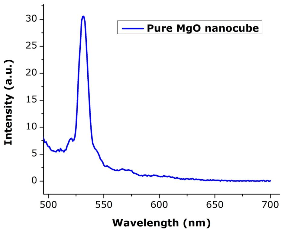
Supplementary Figure S3:- Photoluminescence spectrum when excited at 495 nm of pure MgO nanocube prepared via hydrothermal method.
