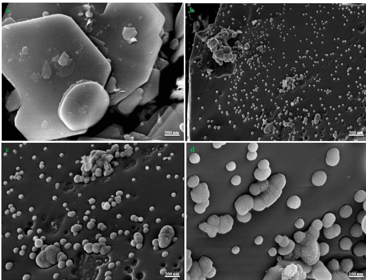
Fig.S1. FESEM images of: (a) pristine MoS<sub>2</sub>, (b) - (d) SnO<sub>2</sub>-decorated MoS<sub>2</sub> nanocomposite, (e) AFM image, (f) line profile and (g) Histogram of nanocomposite.
