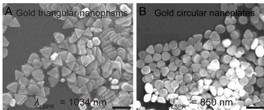
**Figure S4.** Morphologic changes of the GTNPs during the exposing process. Scanning electron microscope (SEM) images taken from the GTNPs (A) before and (B) after being exposed to O<sub>3</sub> (75 ppm) for 60 min with their plasmon modes shifted from 1034 nm to 850 nm. The sharp corners of GTNPs were gradually rounded to form circular nanoplates but the plate-like morphology was preserved. The scale bars are 150 nm.
