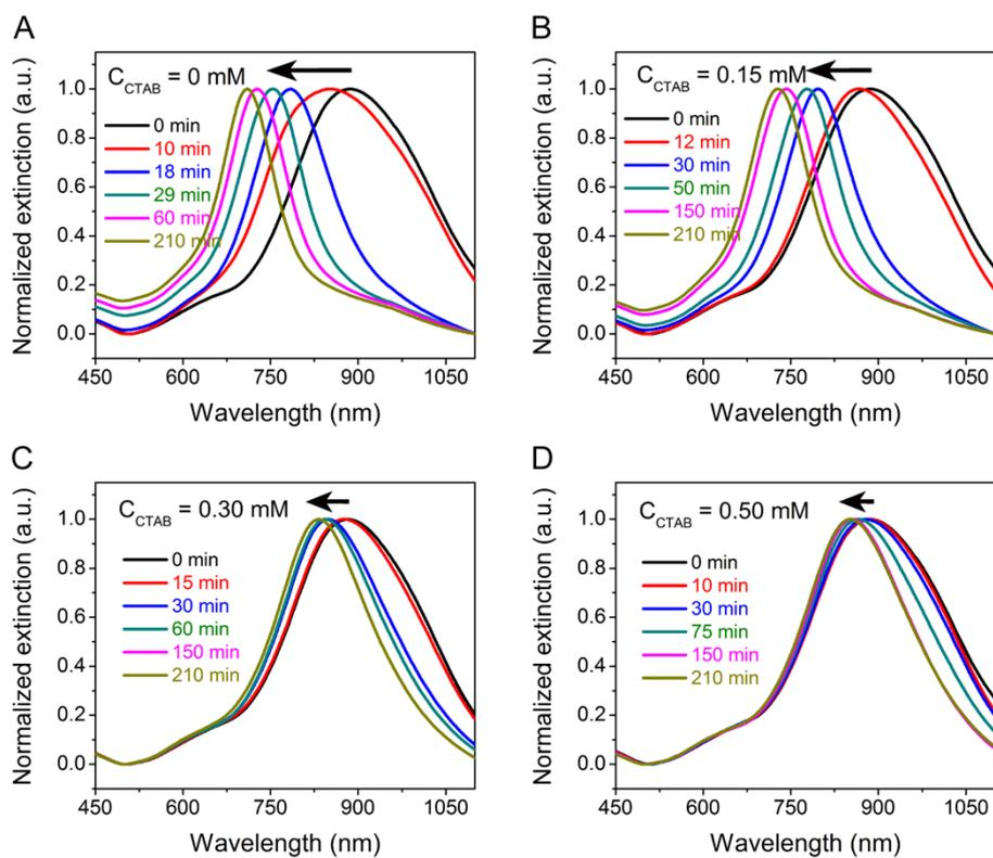
**Figure S5.** The rates of the plasmon mode shifts of GTNPs with different concentrations of CTAB in the suspension. Normalized UV-vis extinction spectra taken from GTNPs exposed to  $O_3$  (~0.08 ppm) with the concentrations of CTAB in the suspension: (A) 0 mM; (B) 0.15 mM; (C) 0.30 mM; (D) 0.50 mM.
