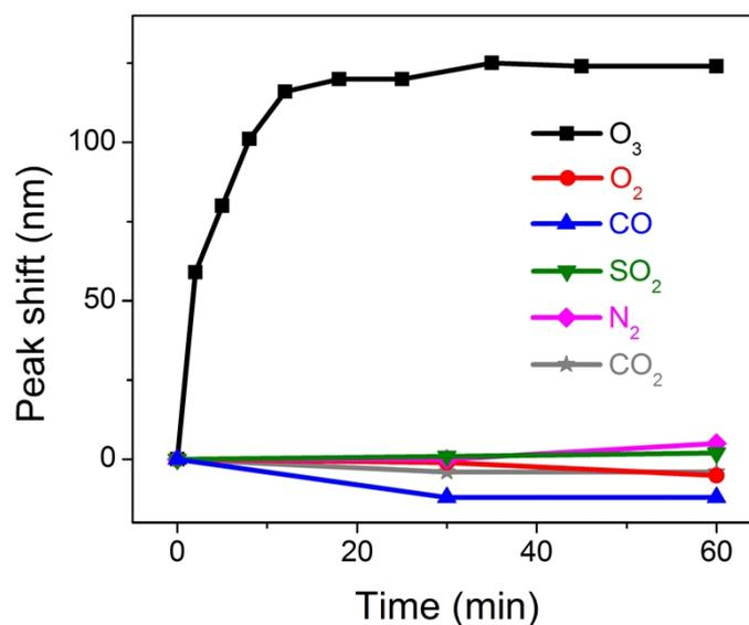
**Figure S2.** The influence of different types of gases in air on the plasmon mode shifts of GTNPs. The plasmon mode shifts of GTNPs as a function of time after exposure to different
