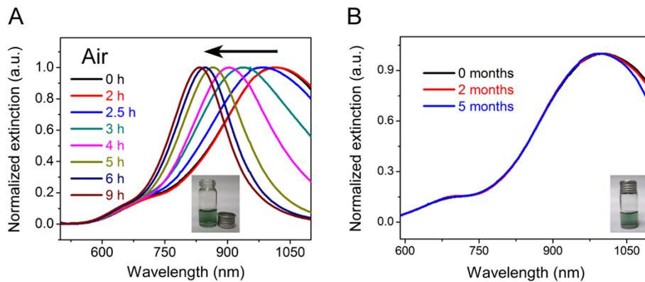
**Figure S1.** (A) Normalized UV-vis absorption spectra taken from solution exposed to air. Inset: photograph of sample exposed to air. The longitudinal plasmon band shifts from 1021 nm to 832 nm in 9 h. (B) Time-dependent normalized UV-vis extinction spectra of GTNPs suspension which was sealed in a bottle for several months. Inset: photograph of suspension sealed in a bottle. The plasmon mode of GTNPs suspension almost didn't shift.
