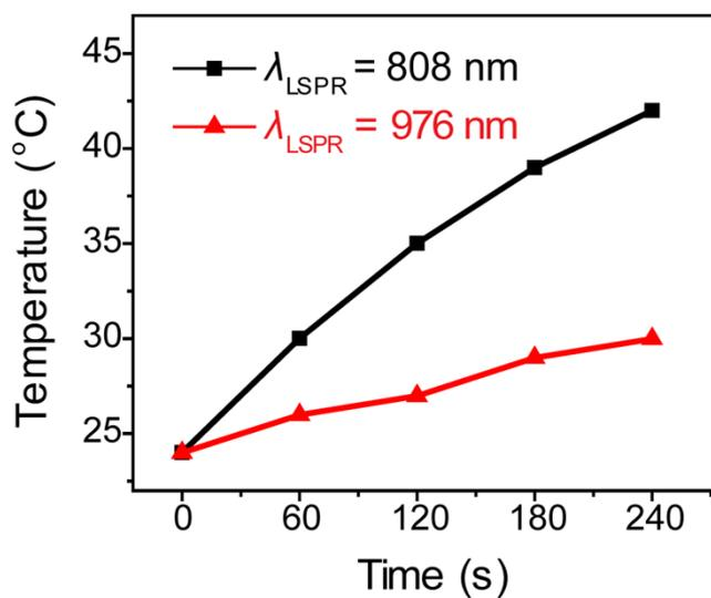
**Figure S9.** The temperature of the center of the channel loaded on with GTNPs obtained plasmon modes of 808 nm (the black line) and 976 nm (the red line) under radiation of a 808 nm laser.
