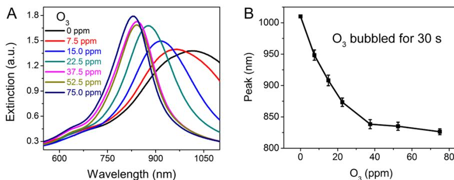
**Figure S3.** The effect of ozone with different concentrations on the plasmon mode shifts of GTNPs. (A) UV-vis extinction spectra of the GTNPs suspensions after exposing to different concentrations of O<sub>3</sub> for 30 s. (B) The concentration-dependent plasmon mode shifts of the GTNPs suspensions corresponding to (A).
