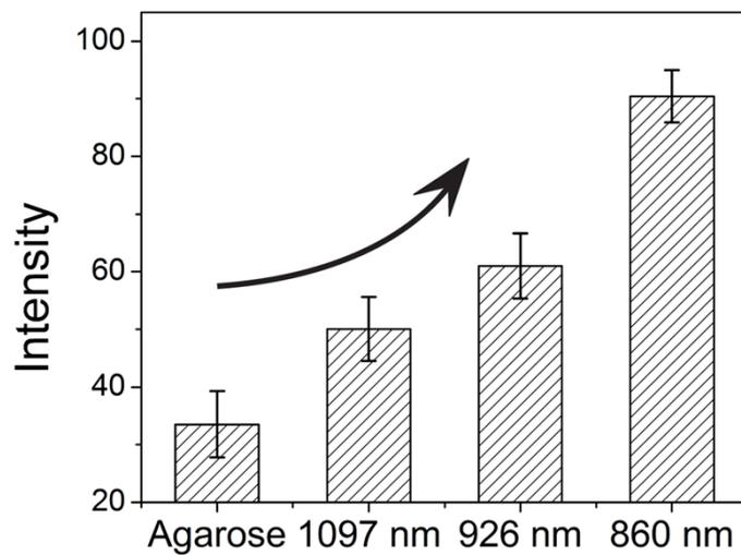
**Figure S8.** Enhancement of OCT signal using GTNPs with different plasmon modes. The signal intensities of agarose gel and GTNPs-agarose phantoms containing GTNPs before ( $\lambda_{\text{LSPR}} = 1097$  nm) and after ( $\lambda_{\text{LSPR}} = 926$  nm and 860 nm) tuning the process were measured by an 840-nm OCT system. We employed an area of 100  $\mu\text{m}$  (width)  $\times$  25  $\mu\text{m}$  (height) for intensity calculation; the
