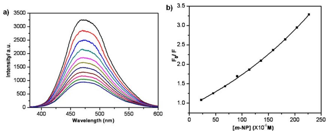
**Fig. S15** (a) Emission spectra ( $\lambda_{\text{ex}} = 350 \text{ nm}$ ) of **1a** ( $4.5 \times 10^{-6} \text{ M}$ ) in presence of *m*-NP at various concentration (0, 5, 10, 15, 20, 25, 30, 35, 40, 45 and 50 equiv.). (b) The nonlinear curve-fitting for the quenching constant of **1a** with *m*-NP.
