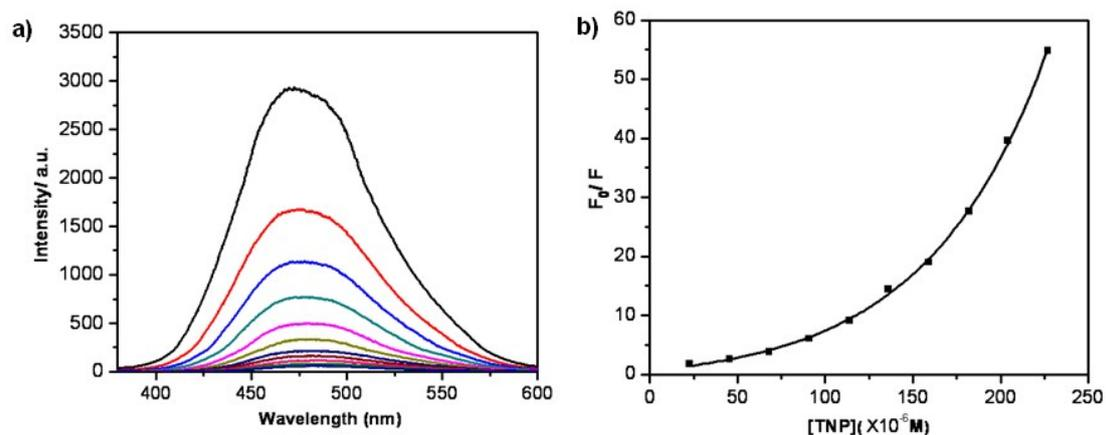
**Fig. S11** (a) Emission spectra ( $\lambda_{\text{ex}} = 350$  nm) of **1a** ( $4.5 \times 10^{-6}$  M) in presence of TNP at various concentration (0, 5, 10, 15, 20, 25, 30, 35, 40, 45 and 50 equiv.). (b) The nonlinear curve-fitting for the quenching constant of **1a** with TNP.
