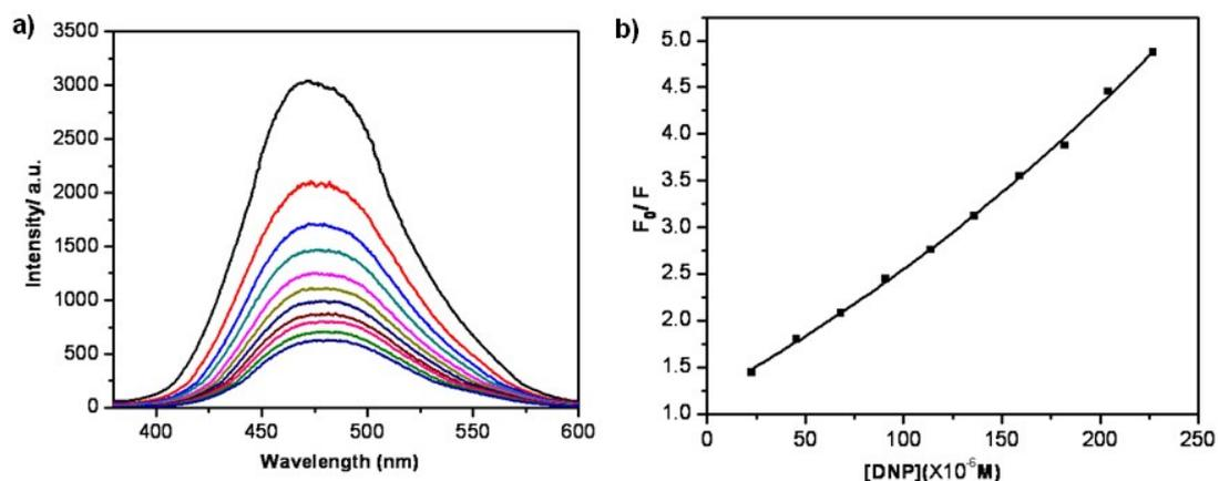
**Fig.S12** (a) Emission spectra ( $\lambda_{\text{ex}} = 350$  nm) of **1a** ( $4.5 \times 10^{-6}$  M) in presence of DNP at various concentration (0, 5, 10, 15, 20, 25, 30, 35, 40, 45 and 50 equiv.). (b) The nonlinear curve-fitting for the quenching constant of **1a** with DNP.
