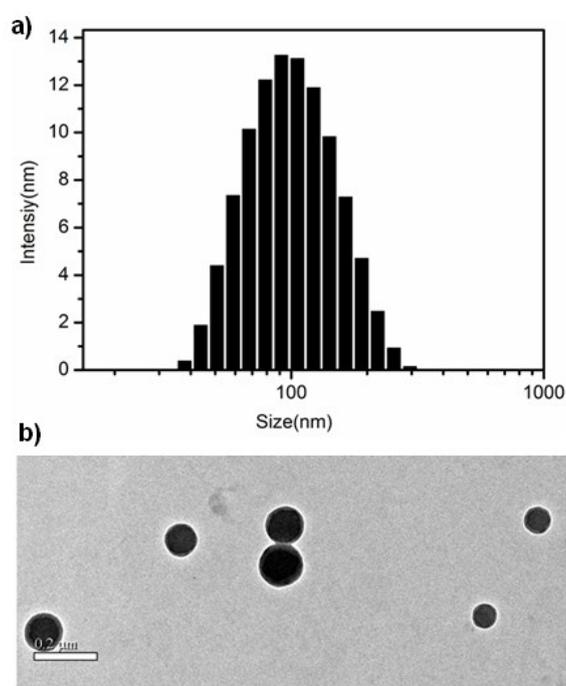
**Fig.S10** The hydrodynamic size (a) and TEM image (b) of **1a** in water/THF (95/5) with concentration of 0.1 mg/mL.
