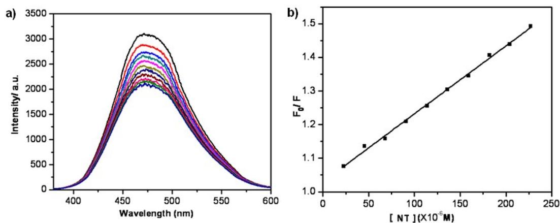
**Fig. S16** (a) Emission spectra ( $\lambda_{\text{ex}} = 350 \text{ nm}$ ) of **1a** ( $4.5 \times 10^{-6} \text{ M}$ ) in presence of NT at various concentration (0, 5, 10, 15, 20, 25, 30, 35, 40, 45 and 50 equiv.). (b) The nonlinear curve-fitting for the quenching constant of **1a** with NT.
