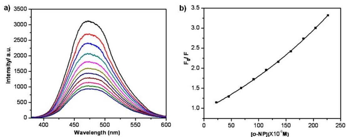
**Fig. S14** (a) Emission spectra ( $\lambda_{\text{ex}} = 350 \text{ nm}$ ) of **1a** ( $4.5 \times 10^{-6} \text{ M}$ ) in presence of *o*-NP at various concentration (0, 5, 10, 15, 20, 25, 30, 35, 40, 45 and 50 equiv.). (b) The nonlinear curve-fitting for the quenching constant of **1a** with *o*-NP.
