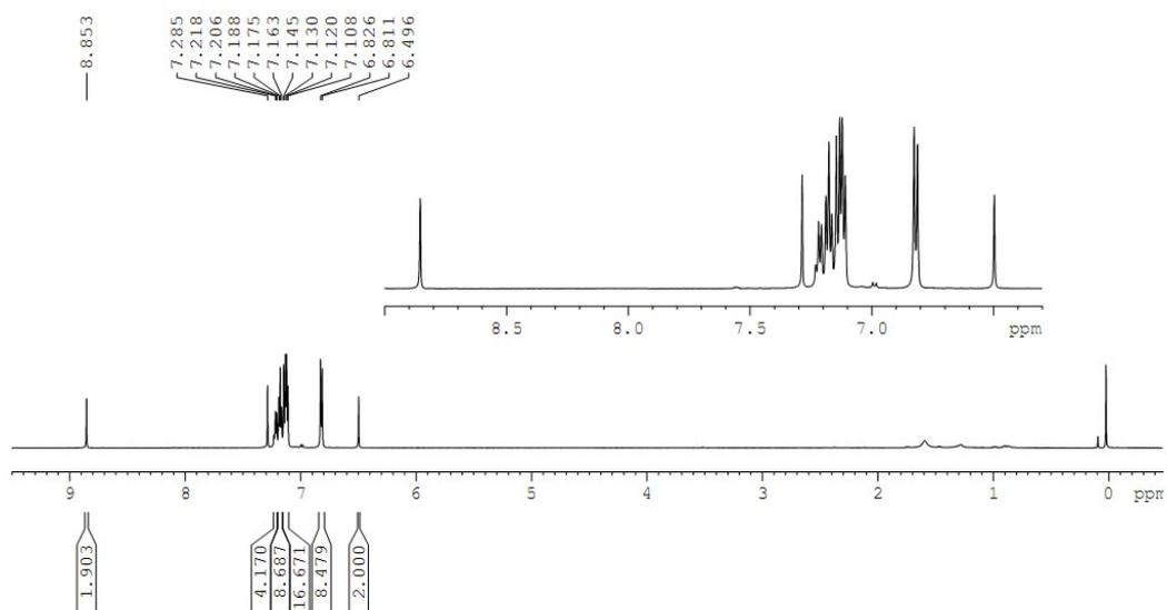
**Fig. S3**  $^1\text{H}$  NMR spectrum (600 MHz,  $\text{CDCl}_3$ ) of **1b**.
