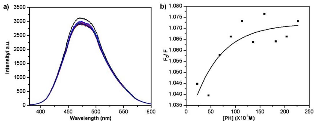
**Fig. S19** (a) Emission spectra ( $\lambda_{\text{ex}} = 350 \text{ nm}$ ) of **1a** ( $4.5 \times 10^{-6} \text{ M}$ ) in presence of PH at various concentration (0, 5, 10, 15, 20, 25, 30, 35, 40, 45 and 50 equiv.). (b) The nonlinear curve-fitting for the quenching constant of **1a** with PH.
