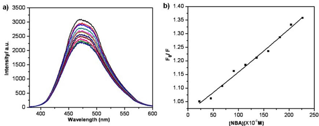
**Fig. S17** (a) Emission spectra ( $\lambda_{\text{ex}} = 350 \text{ nm}$ ) of **1a** ( $4.5 \times 10^{-6} \text{ M}$ ) in presence of NBA at various concentration (0, 5, 10, 15, 20, 25, 30, 35, 40, 45 and 50 equiv.). (b) The nonlinear curve-fitting for the quenching constant of **1a** with NBA.
