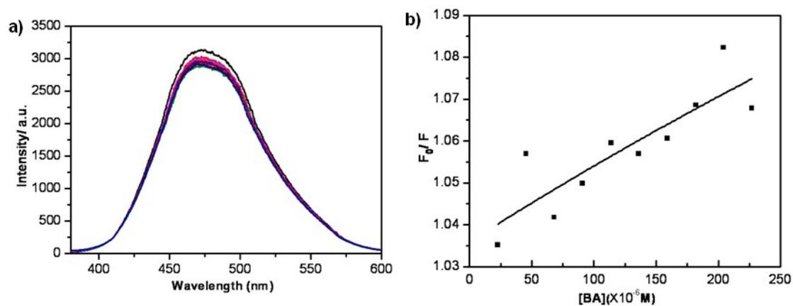
**Fig S18** (a) Emission spectra ( $\lambda_{\text{ex}} = 350 \text{ nm}$ ) of **1a** ( $4.5 \times 10^{-6} \text{ M}$ ) in presence of BA at various concentration (0, 5, 10, 15, 20, 25, 30, 35, 40, 45 and 50 equiv.). (b) The nonlinear curve-fitting for the quenching constant of **1a** with BA.
