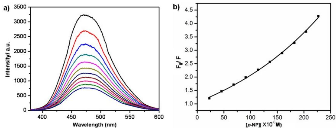
**Fig. S13** (a) Emission spectra ( $\lambda_{\text{ex}} = 350 \text{ nm}$ ) of **1a** ( $4.5 \times 10^{-6} \text{ M}$ ) in presence of *p*-NP at various concentration (0, 5, 10, 15, 20, 25, 30, 35, 40, 45 and 50 equiv.). (b) The nonlinear curve-fitting for the quenching constant of **1a** with *p*-NP.
