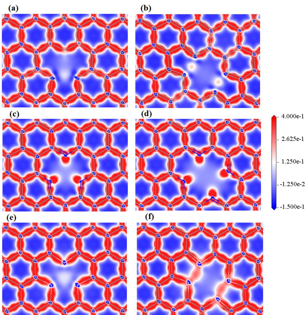
**Fig S 1** Deformation electron density for six V1, (a); V2, (b); VN1, (c); VN2, (d); VB1, (e) and VB2 (f). The red color represents electron accumulation, while the blue color represents electron depletion. The intensity of color depends on the amount of electron change: the darkest red marks the most accumulation; the darkest blue marks the most depletion. (For interpretation of the references to color in this figure legend, the reader is referred to the web version of this article.)
