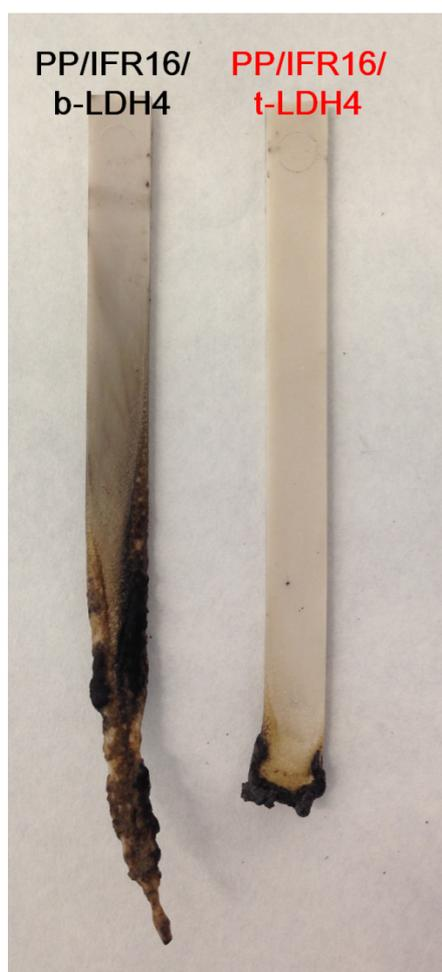
**Fig. S3.** Digital photos of the sample bars after LOI tests.
