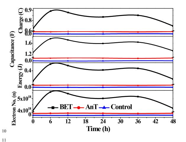
12 Sfig1: Charge, Capacitance, Energy and No of electrons for BET, AnT and Control13 operations
