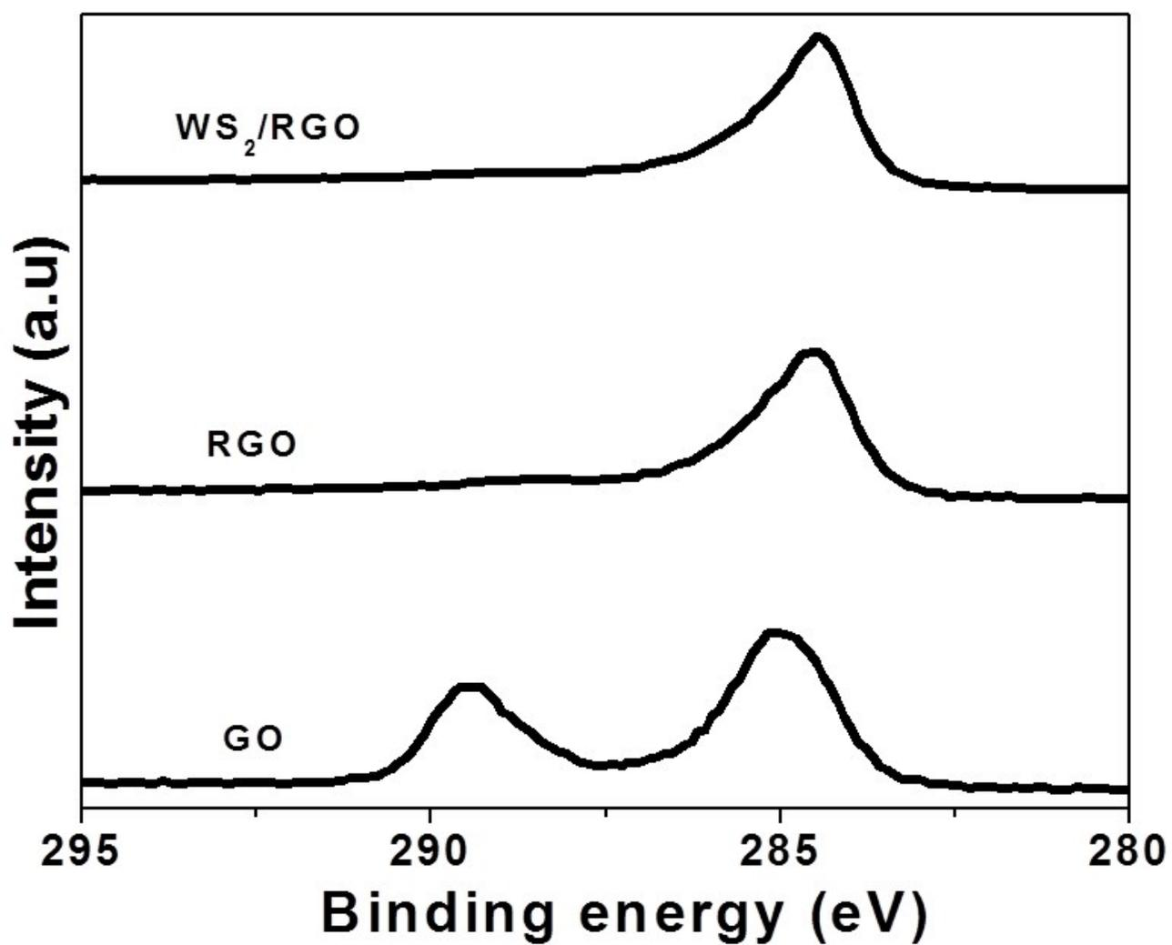
Figure S9: Comparative XPS data for GO, rGO, rGO-WS<sub>2</sub>.
