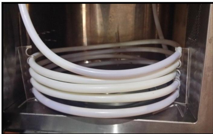
Fig. 2. Teflon coil tube inside microwave cavity
