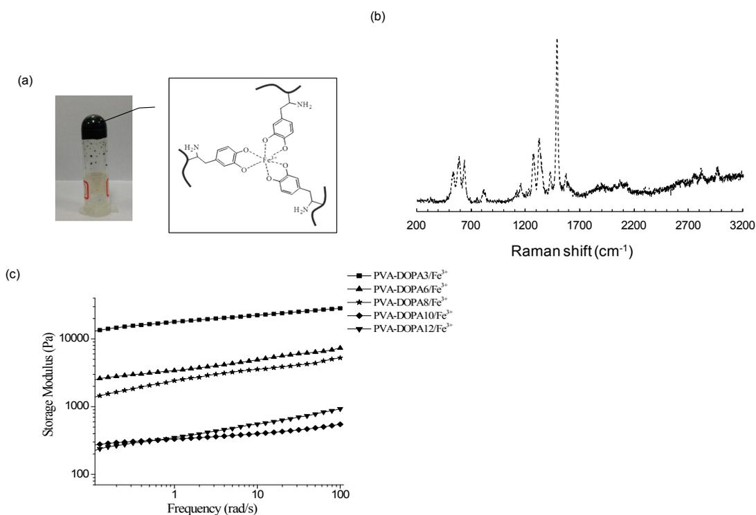
**Figure S3.** (a) Photo image of the PVA-DOPA/ $\text{Fe}^{3+}$  hydrogel in pH 9. (b) Resonance Raman spectrum of the PVA-DOPA3/ $\text{Fe}^{3+}$  complex hydrogel obtained with 532 nm excitation. (c) Frequency sweep of the PVA-DOPA/ $\text{Fe}^{3+}$  hydrogels in pH 9 (25 °C,
