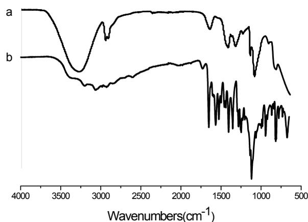
Figure S1. FTIR spectra of PVA (a) and PVA-DOPA12 (b).
