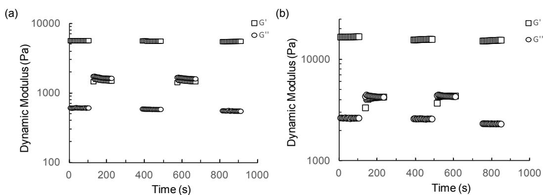
**Figure S4.** Storage moduli  $G'$  and loss moduli  $G''$  of the PVA-DOPA3 hydrogel in pH 3 (a) and pH 12 (b) from continuous strain sweep with alternate small oscillation force at 1% of strain and at 100% of strain.
