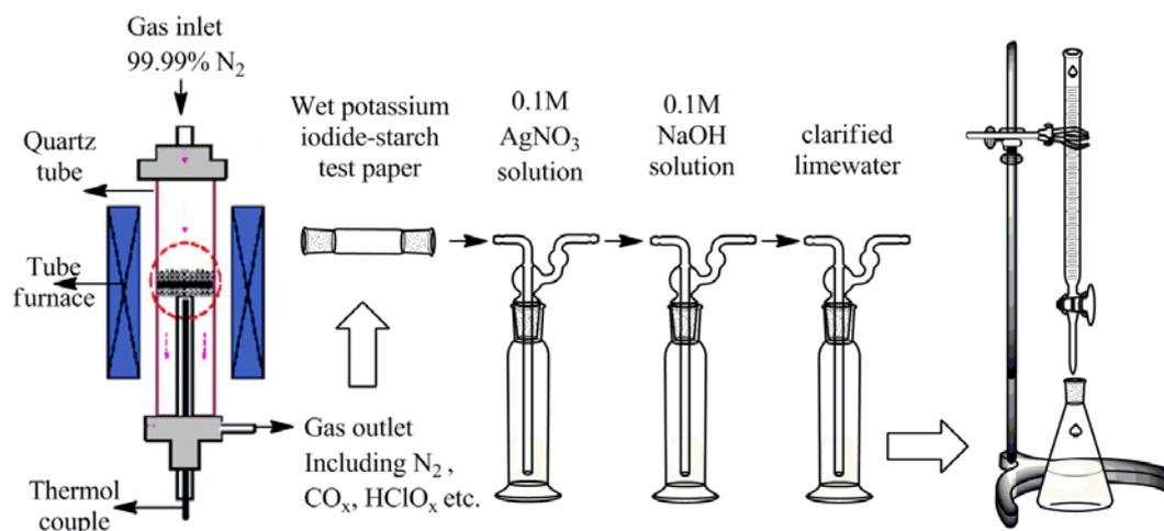
**Scheme S1** In situ chemical absorbing and analyzing of the gas released in the reduction process.
