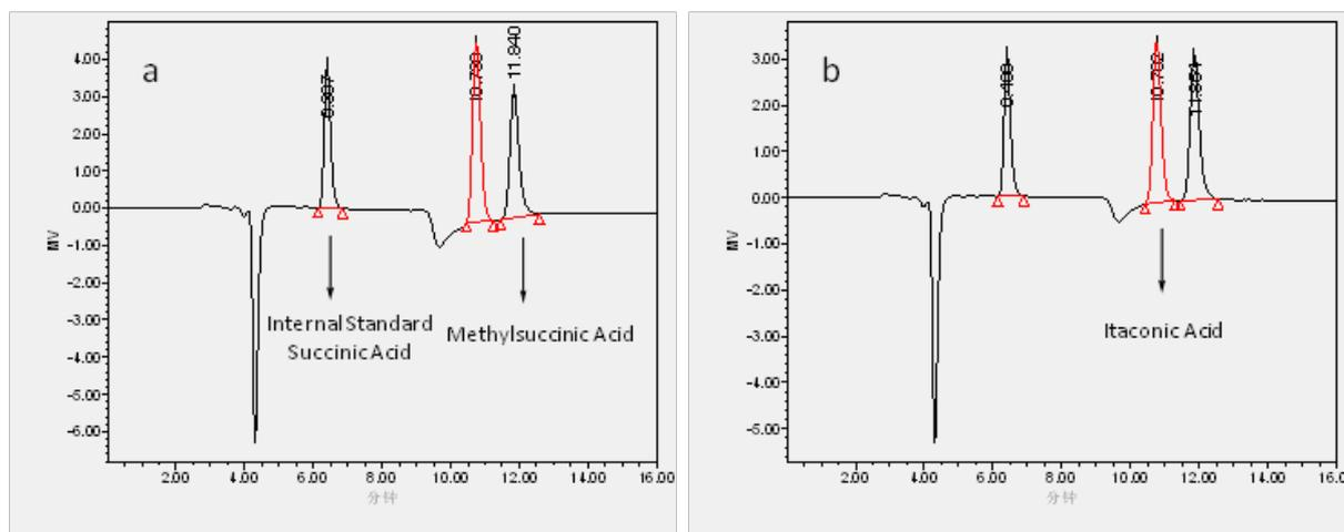
**Fig. S5** HPLC profiles of products detection of the ninth recycling reactions with catalysts Ru/AC-C (a) and Ru/AC-H (b)
