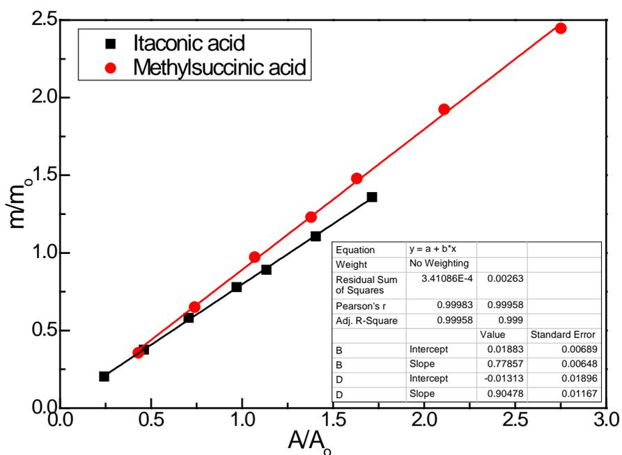
Fig. S4 Standard curve graphs of itaconic acid and methylsuccinic acid using RID detector
