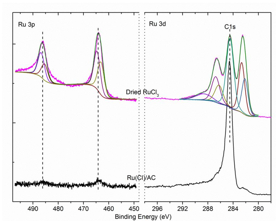
**Fig. S3** XPS spectra of Ru3p and Ru3d transition in samples of dried RuCl<sub>3</sub>, Ru(Cl)/AC
