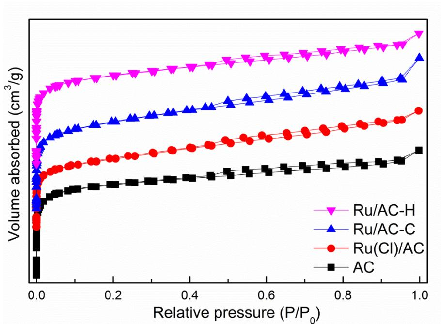
Fig. S1 N<sub>2</sub> physisorption of supports and catalysts
