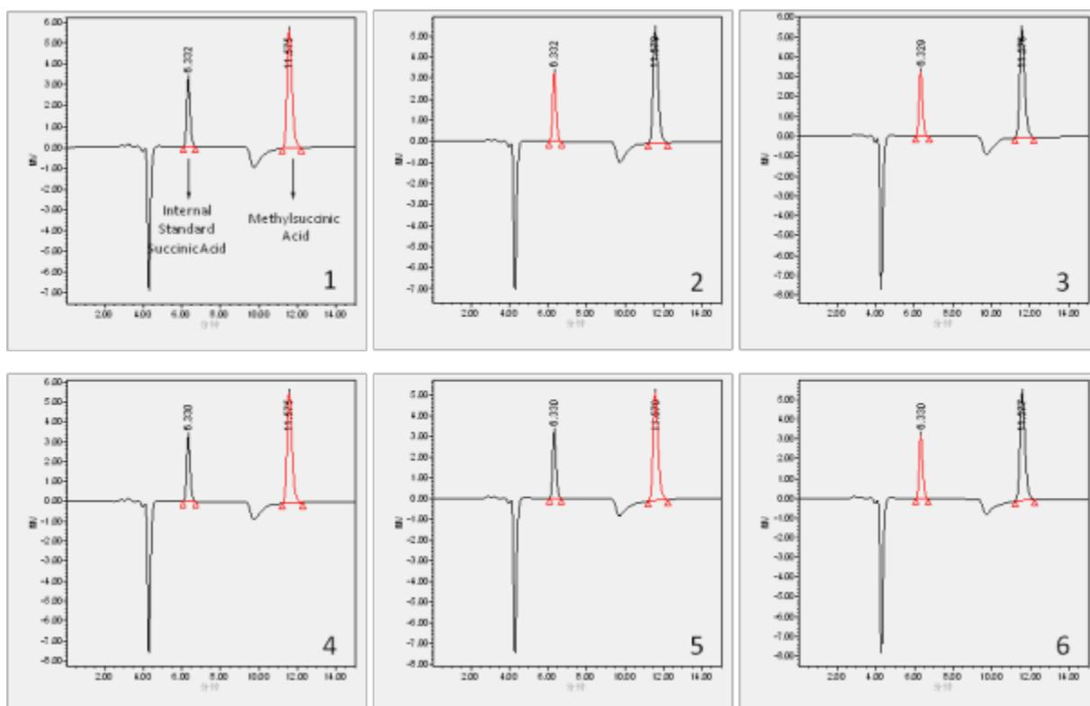
**Fig. S6** HPLC profiles of products detection for Ru/AC-C in 6 recycle times
