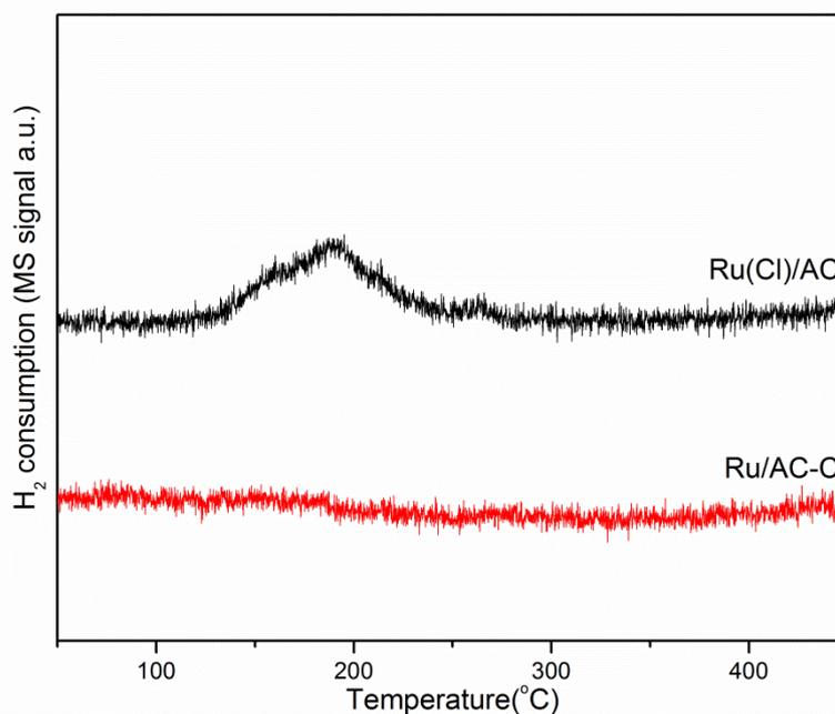
Fig. S2 MS profiles of H<sub>2</sub>-TPR tests of Ru(Cl)/AC and Ru/AC-C in Fig.3
