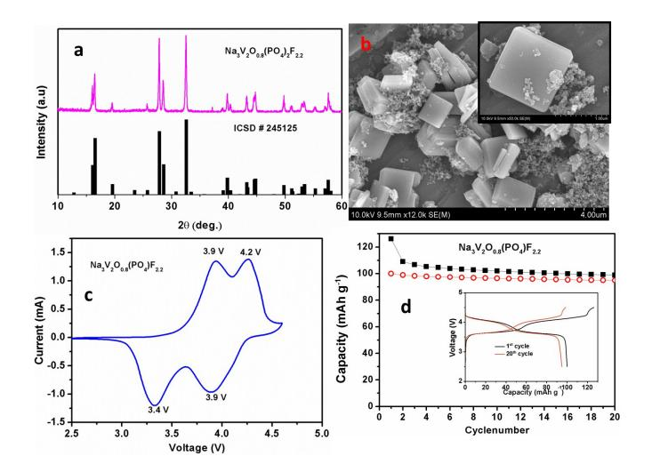
Fig. S2 (a) XRD patterns, (b) SEM images and (c) Cyclic voltammetry for the prepared  $Na_3V_2O_{2x}$  (PO<sub>4</sub>)<sub>2</sub>F<sub>3-2x</sub> sample. (d) Half-cell galvanostatic cycling performance at 0.1C rate up to 20 cycles.
