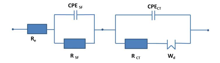
Fig. S1 An equivalent circuit for analysis of the EIS results.
