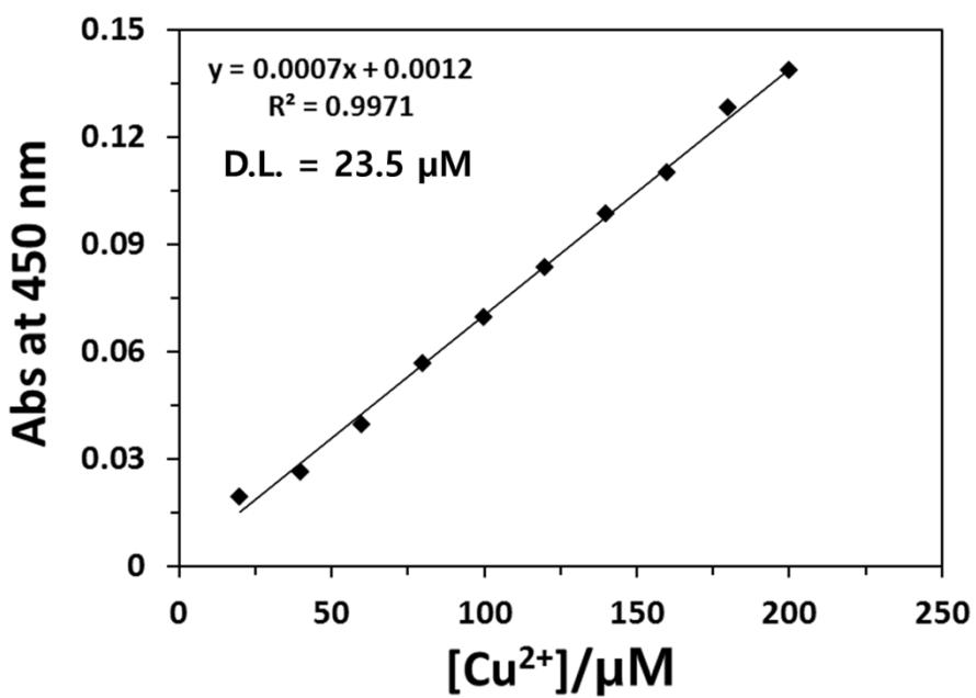
**Fig. S4** Detection limit of **1** (20  $\mu\text{M}$ ) for Cu<sup>2+</sup> through change of absorbance at 450 nm.
