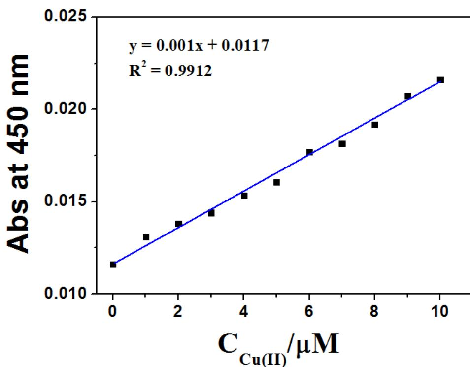
**Fig. S6** Absorbance (at 450 nm) of **1** as a function of Cu<sup>2+</sup> concentration ([**1**] = 20  $\mu\text{mol/L}$  and [Cu<sup>2+</sup>] = 0 - 10  $\mu\text{mol/L}$ ).
