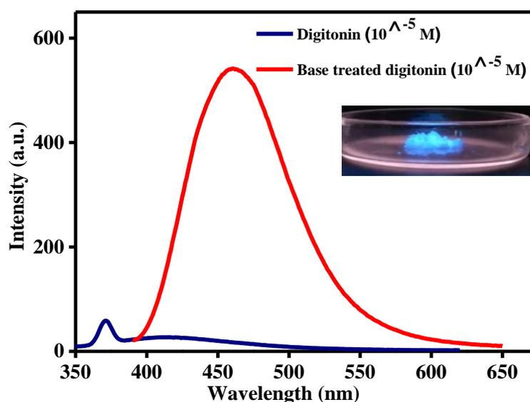
**Figure S2:** PL emission spectra of digitonin (a) and base treated digitonin (b) at a concentration of  $10^{-5}$  M. Inset: photographs of solid state emission of base treated digitonin under hand held UV light ( $\lambda_{ex}$ : 365 nm).
