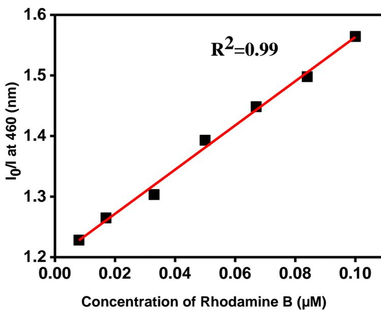
**Figure S12:** Stern-Volmer plot of  $I_0/I$  versus concentration of quencher for white light emitting base treated digitonin-Rhodamine mixture.
