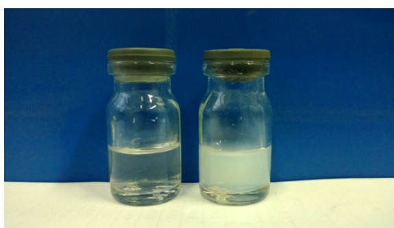
Fig.S2 The image of 3mg/mL free copolymer (1) solution at 0°C and 35°C.
