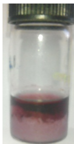
Figure S6. Retro-gradation of starch was performed by freezing and thawing. The bottom of the bottle showed retrograded starch (light pink color) with AuNP while dark ruby red color showed AuNP suspension.
