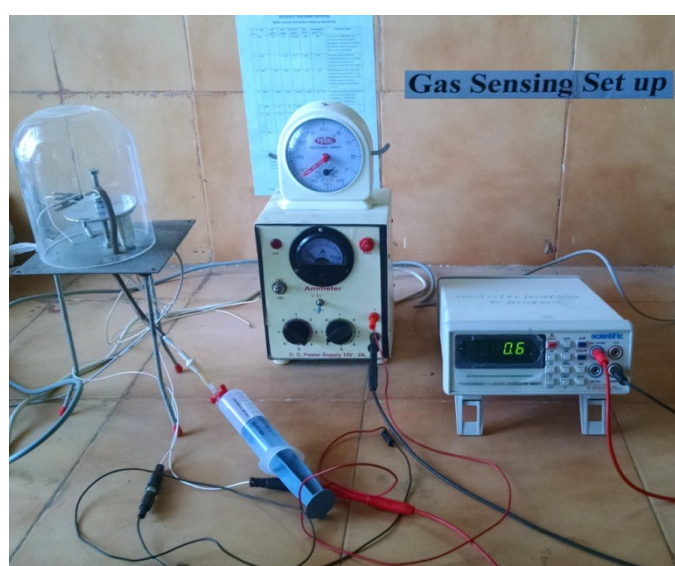
Figure S4. Photographic representation of a two-probe gas sensing setup at laboratory
