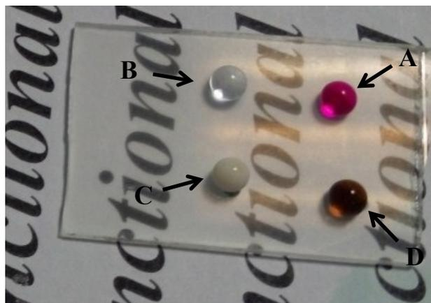
Fig. S2. Digital image of coating A with water (A), ethylene glycol (B), milk (C) and vinegar (D) droplets on its surface. Rhodamine 6G was added in water for easy differentiation.
