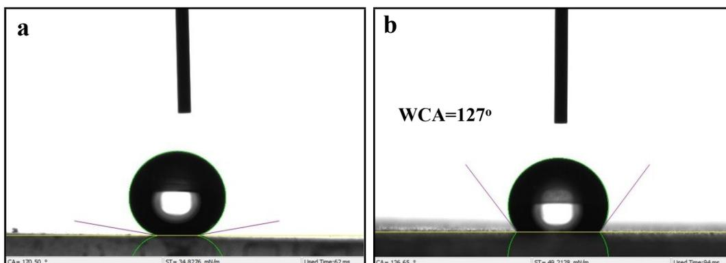
Fig. S5. Water Contact angles of coatings B (a) and C (b).
