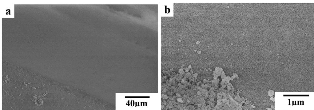
Fig. S4. SEM (a) and magnified SEM (b) images of coating B after 2H pencil scratching test.
