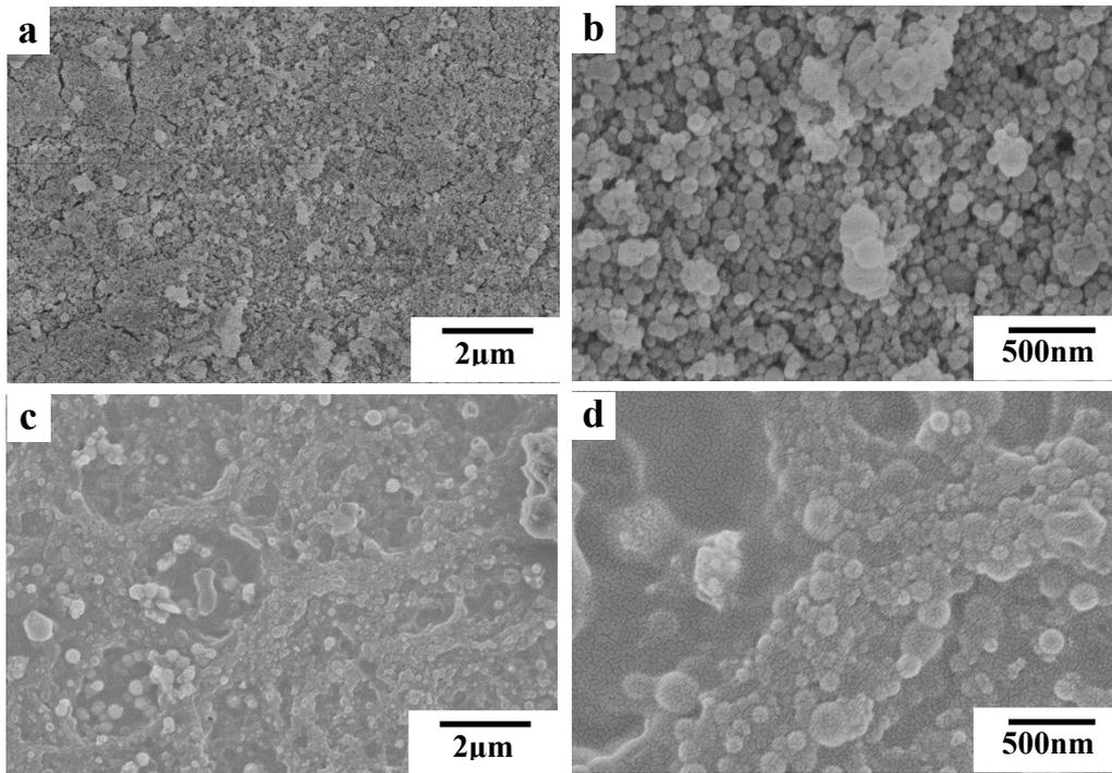
Fig. S3 SEM images showing the surface morphologies of coatings B (a, b) and C (c, d).
