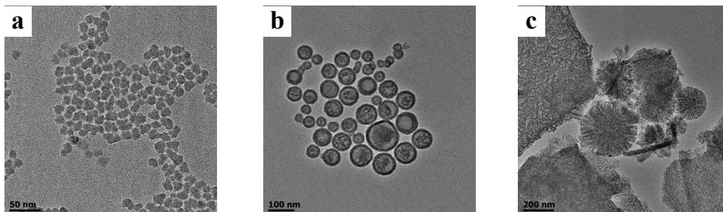
Fig. S1. TEM images of 20 nm silica nanoparticles (a), silica hollow nanospheres (b) and silica nanosheets (c).
