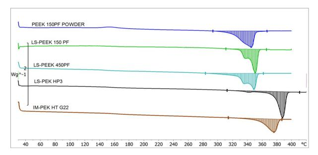
Although the PEEK 150 powder does not show distinguishable double melting peaks as Laser sintered 150PF, it has a broad melting peak with non-symmetric shape. The broad melting range suggests the possible presents of highly overlapped melting peaks. The same result is observed in the injection moulded PEK HT G22.
