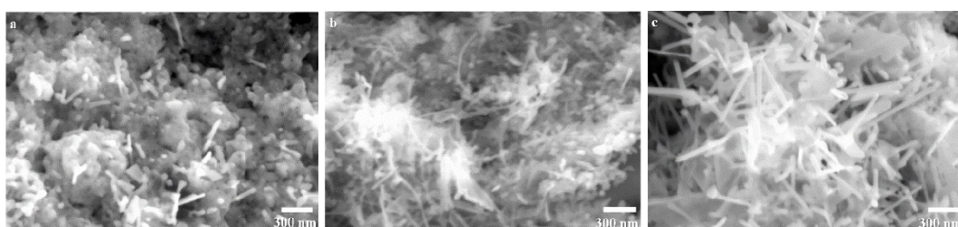
Figure S5. SEM images of Cu materials synthesized with 22 \mu L of HNO 3 at 17°C for different reaction time: (a) 3h; (b) 6h; (c) 10h. The concentration of CuCl 2 and CTAC is 5 mM and 1.8 mM, respectively.
