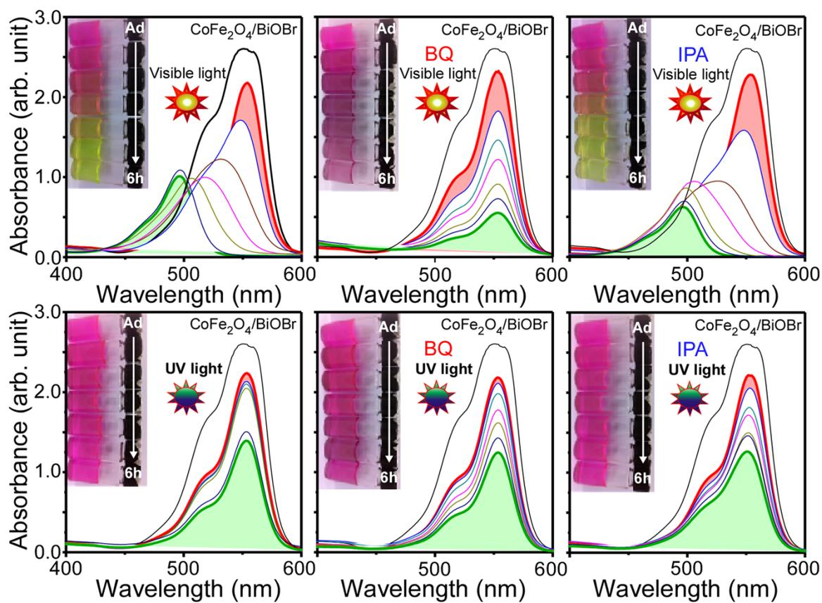
**Figure S5.** Adsorption (in dark) and photodegradation (under UV and visible lights) tests of RhB (20 mg/L, 100 mL) over 25 mg CoFe<sub>2</sub>O<sub>4</sub>/BiOBr microflowers. The insets show the corresponding photographs displaying a change in dye color with the photodegradation time.
