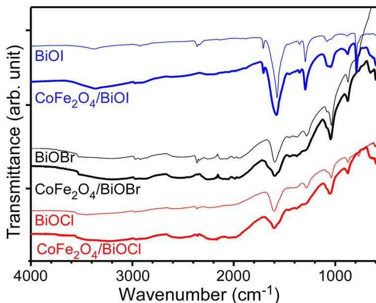
**Figure S2.** FT-IR spectra of the  $\text{CoFe}_2\text{O}_4/\text{BiOX}$  (X= Cl, Br and I) and  $\text{BiOX}$  microflowers.
