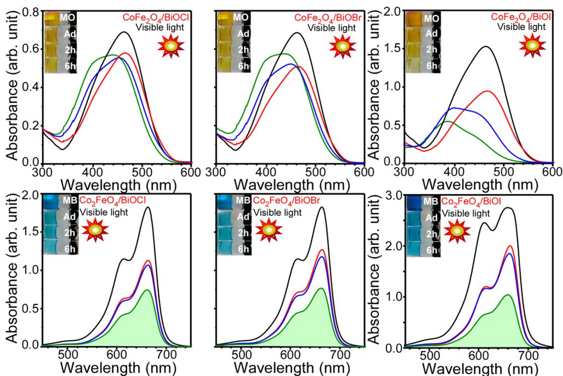
**Figure S6.** Adsorption (in dark) and photodegradation (under visible lights) tests of MO and MB (50 mL) over 25 mg  $\text{CoFe}_2\text{O}_4/\text{BiOX}$  microflowers. Dye concentrations were 10 mg/L for  $\text{CoFe}_2\text{O}_4/\text{BiOCl}$  and  $\text{CoFe}_2\text{O}_4/\text{BiOBr}$ , and 20 mg/L for  $\text{CoFe}_2\text{O}_4/\text{BiOI}$ . The insets show the corresponding photographs displaying a change in the dye color with photodegradation time.
