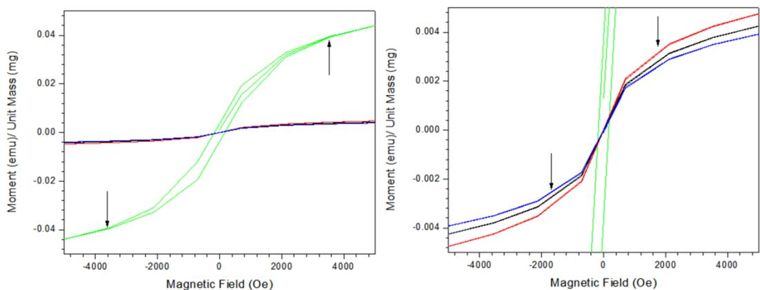
**Figure S3.** Magnified magnetization (M–H) curves for CoFe<sub>2</sub>O<sub>4</sub> NPs (left) and CoFe<sub>2</sub>O<sub>4</sub>/BiOX (X= Cl: red color, Br: black color and I: blue color) microflowers (right) with applied magnetic fields from –4.5 to 4.5 kOe.
