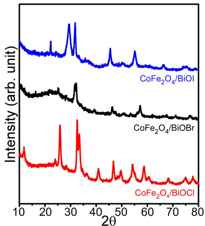
**Figure S7.** Power X-ray diffraction patterns of  $\text{CoFe}_2\text{O}_4/\text{BiOX}$  ( $X = \text{Cl}, \text{Br}$  and  $\text{I}$ ) microflowers after photocatalytic dye degradation experiments.
