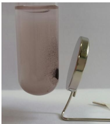
**Figure S4.** Powder sample dispersed in a dye solution is easily attracted by a magnet.
