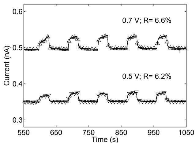
**Fig. S7b:** Current-time measurements under NIR chopped light (60 s dark and 30 s under irradiation,  $\lambda_{\text{exc}} = 980$  nm,  $1 \text{ W/cm}^2$ ) for 6 mol%  $\text{LiYF}_4: \text{Tm}^{3+}, \text{Yb}^{3+}$  UCNP/ $\text{WO}_3$  films deposited on patterned ITO (interelectrode distance 100  $\mu\text{m}$ ), treated at 385  $^\circ\text{C}$ .
