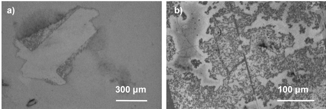
**Fig. S2** Optical microscopy images of 16 mol% UCNP/WO<sub>3</sub> films thermally treated at 385 °C deposited on a) glass and b) SiO<sub>2</sub>.
