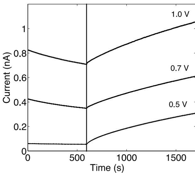
**Fig. S6** Current-time measurements under simulated solar light (power density of  $1 \text{ W/cm}^2$ , irradiation starts at  $t = 600 \text{ s}$ ; before irradiation samples were kept under bias in the dark) for 8 mol% UCNP/ $\text{WO}_3$  films deposited on patterned ITO (interelectrode distance  $100 \mu\text{m}$ ), thermally treated at  $385 \text{ }^\circ\text{C}$ .
