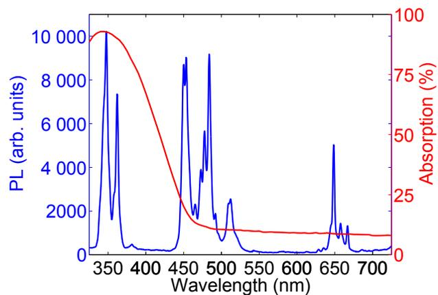
**Fig. S7a:** Absorption spectrum of ca. 1.2  $\mu\text{m}$ -thick  $\text{WO}_3$  films (left y axis) and PL spectrum of  $\text{LiYF}_4: \text{Tm}^{3+}, \text{Yb}^{3+}$  upconverting nanoparticles on glass (right y axis). When excited at  $\lambda_{\text{exc}} = 980$  nm, the UCNP have three emission bands in the visible range, partially overlapping with the spectrum of  $\text{WO}_3$ .
