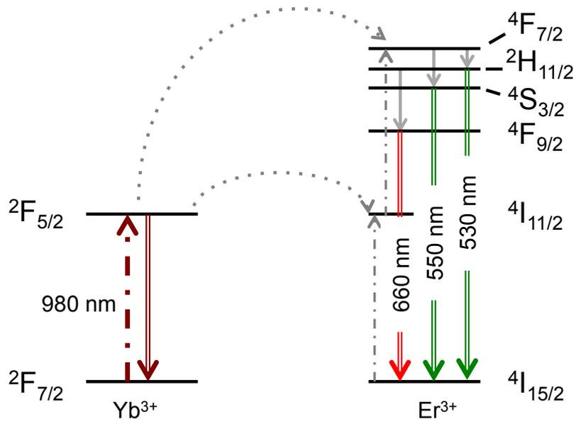
**Fig. S1** Partial  $\text{NaGdF}_4:\text{Er}^{3+}, \text{Yb}^{3+}$  UCNPs energy levels diagram. For the sake of clarity, only the energy levels involved in the upconversion process are shown. Dashed lines are associated with energy absorption, dotted lines are associated with energy transfer, full grey lines are associated with non-radiative processes, and full double lines are associated with radiative processes.
