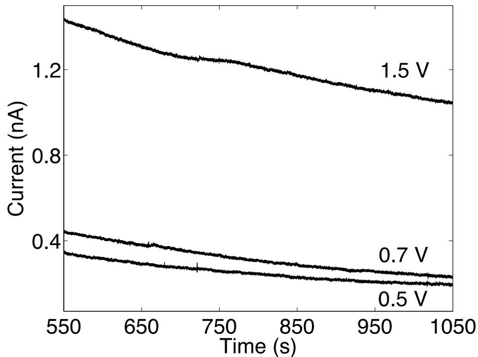
**Fig. S3** Current-time measurements under NIR chopped light ( $\lambda_{\text{exc}} = 980$  nm, power density of 1 W/cm<sup>2</sup>) for films made of 6 mol% UCNP/WO<sub>3</sub> deposited on patterned ITO (interelectrode distance of 100  $\mu\text{m}$ ), thermally treated at 385 °C. Samples were kept under a constant electrical bias for 300 s in ambient light conditions, followed by 300 s in the dark, before chopping the light (60 s in the dark and 30 s under irradiation).
