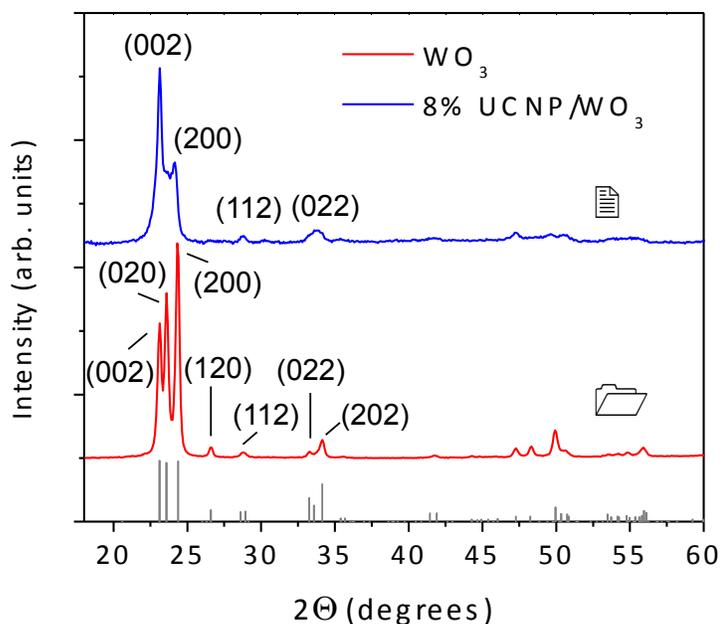
**Fig. S4** XRD measurements of WO<sub>3</sub> (pattern 1) and ~ 8 mol% UCNP/WO<sub>3</sub> thin films deposited on glass and thermally treated at 385 °C (pattern 2).
