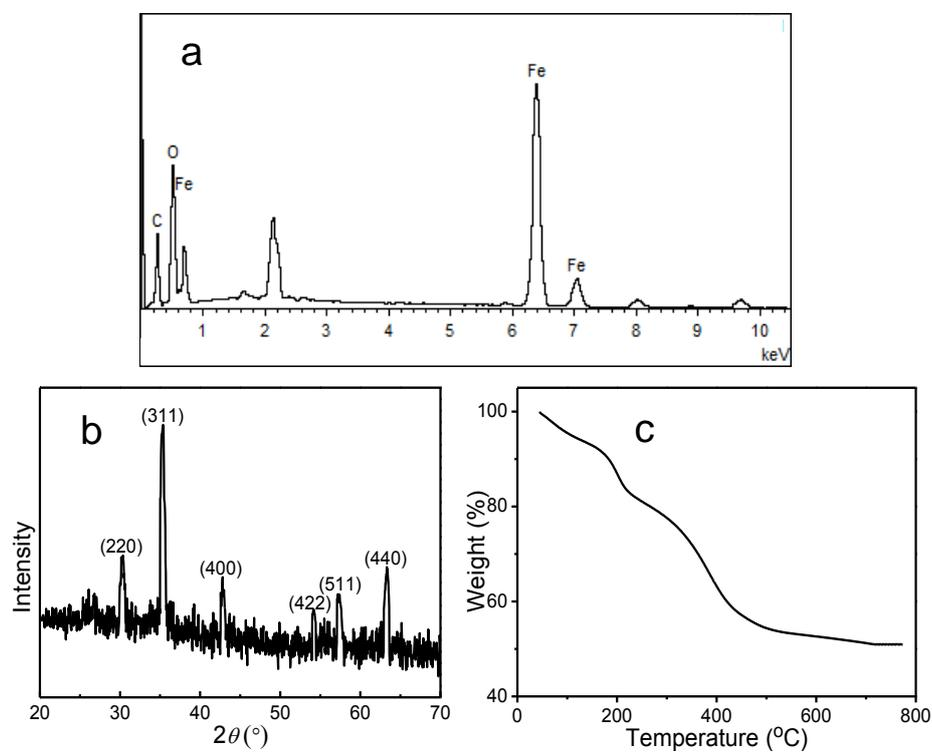
**Fig. S2.** (a) EDS spectrum, (b) XRD pattern and (c) TGA curve of  $\text{Fe}_3\text{O}_4$  nanoparticle-decorated GO.
