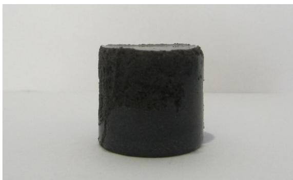
**Fig. S8.** Digital photograph of porous nanoparticle-decorated GO/PMF foam.
