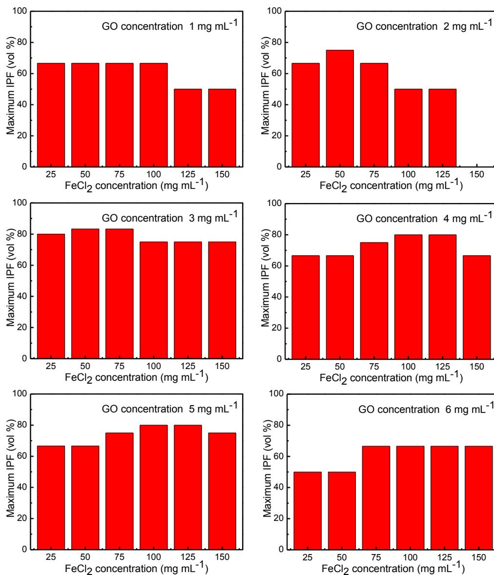
**Fig. S5.** The maximum internal phase fractions (IPFs) of toluene-in-water emulsions prepared with various GO concentrations and FeCl<sub>2</sub> concentrations.
