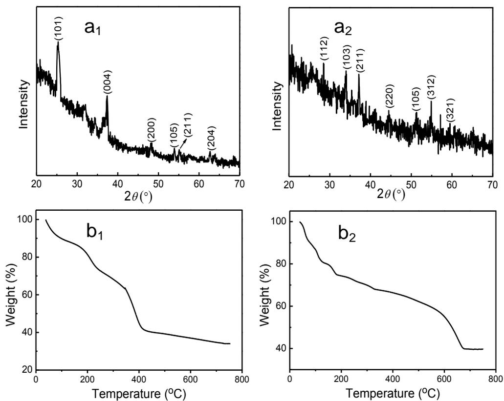
**Fig. S7.** XRD patterns of (a<sub>1</sub>) TiO<sub>2</sub> and (a<sub>2</sub>) Mn<sub>3</sub>O<sub>4</sub> nanoparticle-decorated GO sheets. TGA curves of (b<sub>1</sub>) TiO<sub>2</sub> and (b<sub>2</sub>) Mn<sub>3</sub>O<sub>4</sub> nanoparticle-decorated GO sheets.
