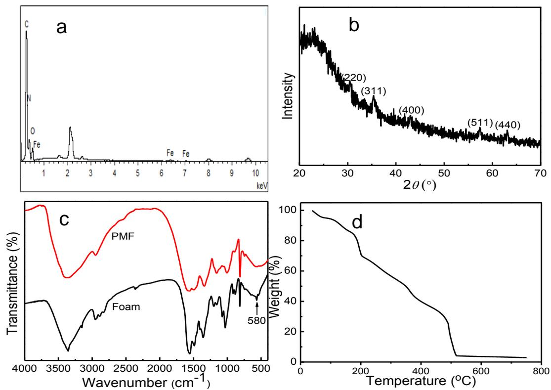
**Fig. S9.** (a) EDS spectrum and (b) XRD pattern of porous Fe<sub>3</sub>O<sub>4</sub> nanoparticle-decorated GO/PMF foam. (c) FTIR spectrum of pure PMF and porous Fe<sub>3</sub>O<sub>4</sub> nanoparticle-decorated GO/PMF foam. (d) TGA curve of porous Fe<sub>3</sub>O<sub>4</sub> nanoparticle-decorated GO/PMF foam.
