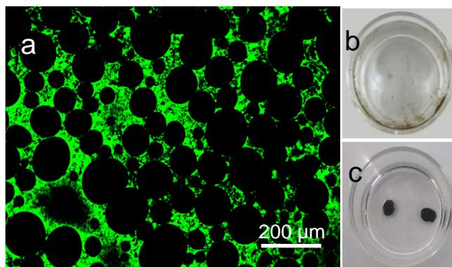
**Fig. S3.** (a) Fluorescence micrograph of toluene-in-water Pickering HIPE stabilized by  $\text{Fe}_3\text{O}_4$  nanoparticle-decorated GO sheets. Digital photographs of drop test of the Pickering HIPE dispersing in (b) water and (c) toluene. The internal phase fraction of Pickering HIPE is 80 vol%.
