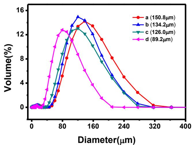
**Fig. S4.** The size distribution graphs of toluene-in-water Pickering HIPEs stabilized by  $\text{Fe}_3\text{O}_4$  nanoparticle-decorated GO sheets formed with different concentration of  $\text{FeCl}_2$ : (a) 18.75, (b) 25, (c) 31.25, and (d) 37.5  $\text{mg mL}^{-1}$ . The GO sheet concentration in aqueous suspension is 3  $\text{mg mL}^{-1}$ . The internal phase fraction of the emulsions is 75 vol%.
