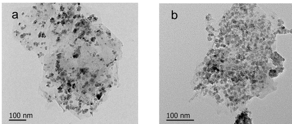
**Fig. S6.** TEM images of (a) TiO<sub>2</sub> and (b) Mn<sub>3</sub>O<sub>4</sub> nanoparticle-decorated GO sheets.
