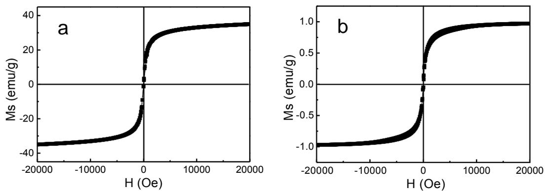
Fig. S1. Magnetization curves of (a) Fe<sub>3</sub>O<sub>4</sub> nanoparticle-decorated GO and (b) porous Fe<sub>3</sub>O<sub>4</sub> nanoparticle-decorated GO/PMF foams.
