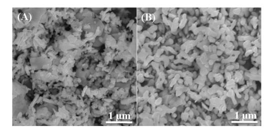
Fig.S1 SEM spectra of nano α-Bi<sub>2</sub>O<sub>3</sub> (A) and β-Bi<sub>2</sub>O<sub>3</sub> (B)
