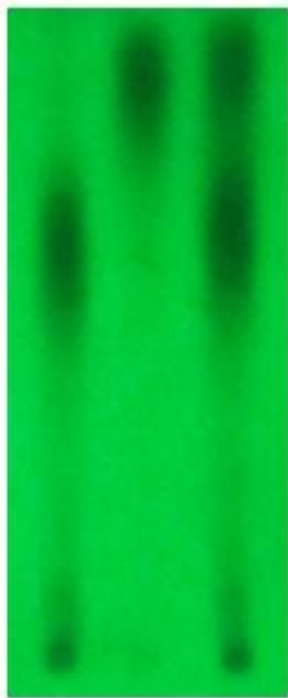
Figure S20. R_f value of 2 (middle), 3 (left), the mixture of 2 and 3 (right) in thin-layer chromatography ( \text{SiO}_2 , PE:DCM:EA = 10:10:1).
