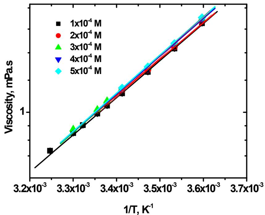
**Fig. S3** Variation of viscosity of 0.12 % (w/v) Triton X 114) with temperature as a function of PMBP concentration in 0.1 M Na-acetate
