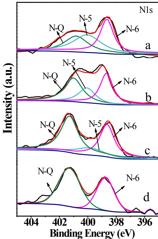
**Figure S4** N1s XPS spectra of (a) S-600 , (b) S-700 , (c) HPNCNTs and (d) S-900 .
