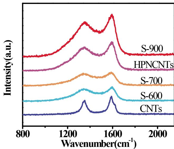
**Figure S2** Raman spectra of pristine CNTs, HPNCNTs, S-600, S-700 and S-900.
