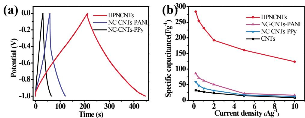
**Figure S5** (a) Galvanostatic charge/discharge curves at  $1 \text{ A g}^{-1}$ . (b) Specific capacitances of HPNCNTs, NC-CNTs-PANI, NC-CNTs-PPy and CNTs electrodes at different current densities.
