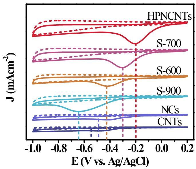
**Figure S6** CV curves in  $\text{N}_2$ -saturated (dashed curves) and  $\text{O}_2$ -saturated (solid curves) solution with a sweep rate of  $50 \text{ mV s}^{-1}$ .
