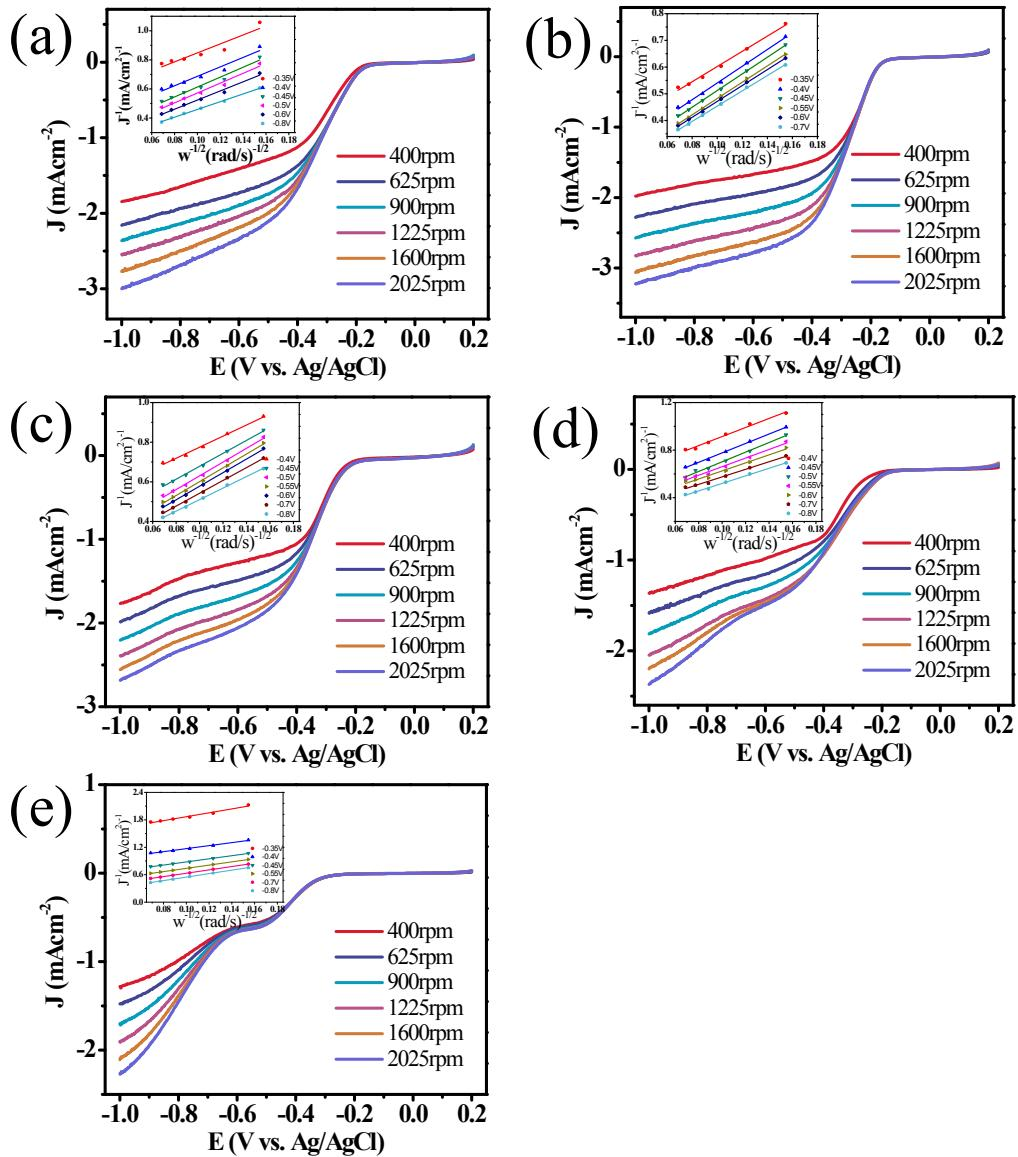
**Figure S7** RDE polarization curves for (a) S-600, (b) S-700, (c) S-900, (d) NCs and (e) CNTs in  $O_2$ -saturated solution at different rotation speeds. Scan rate:  $10 \text{ mV s}^{-1}$ . The inset shows the partial K-L plots derived from the RDE measurements of the sample.
