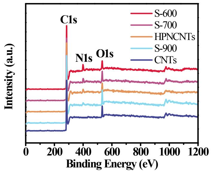
**Figure S3** XPS survey spectra of CNTs and HPNCNTs, S-600, S-700 and S-900.
