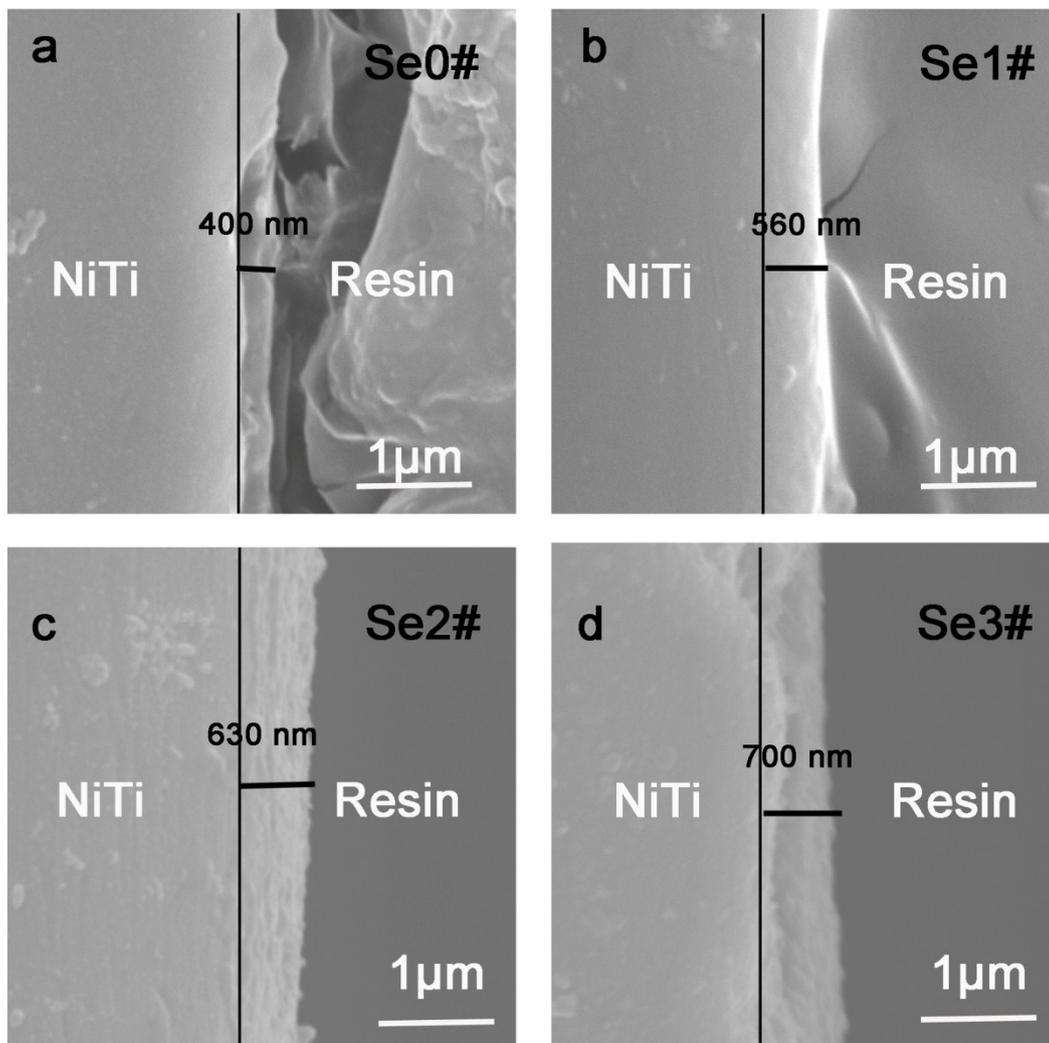
**Fig. S9** SEM images show the cross section of different samples, a: Se0#, b: Se1#, c: Se2#, d: Se3#.
