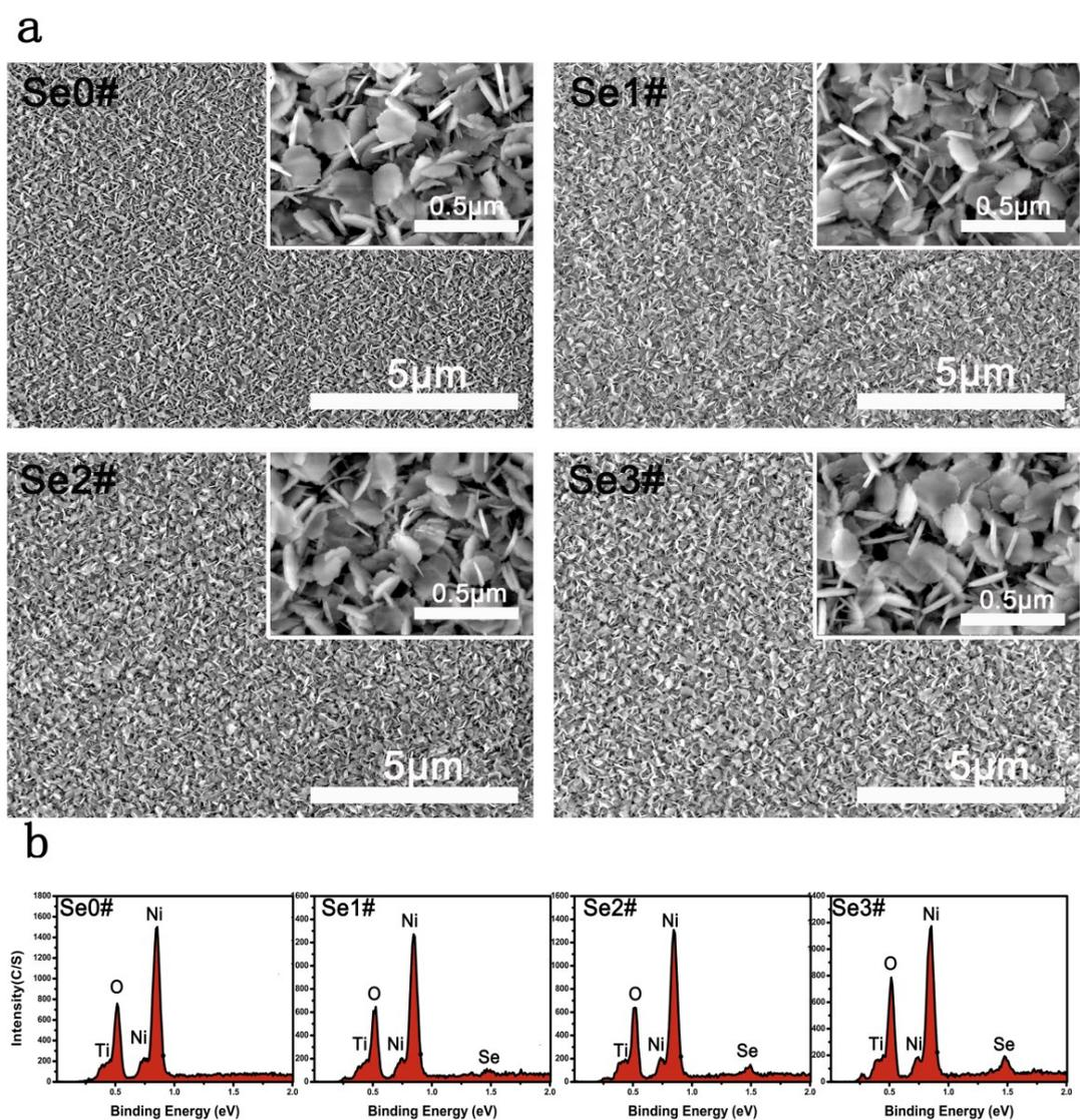
**Fig.S3** SEM images of different samples at low and high magnification (a), and the corresponding EDS patterns (b).
