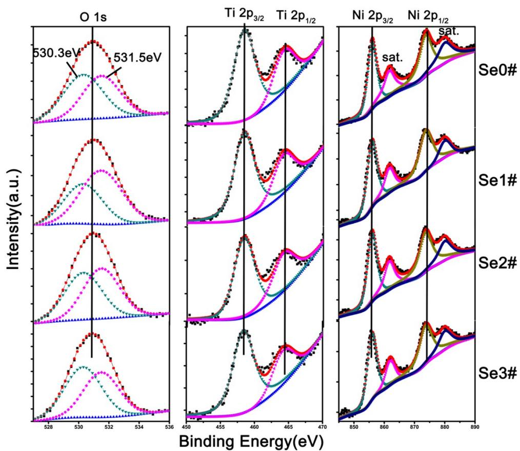
Fig.S2 XPS spectra of O 1s, Ti 2p and Ni 2p in sample Se0#, Se1#, Se2# and Se3# respectively.
