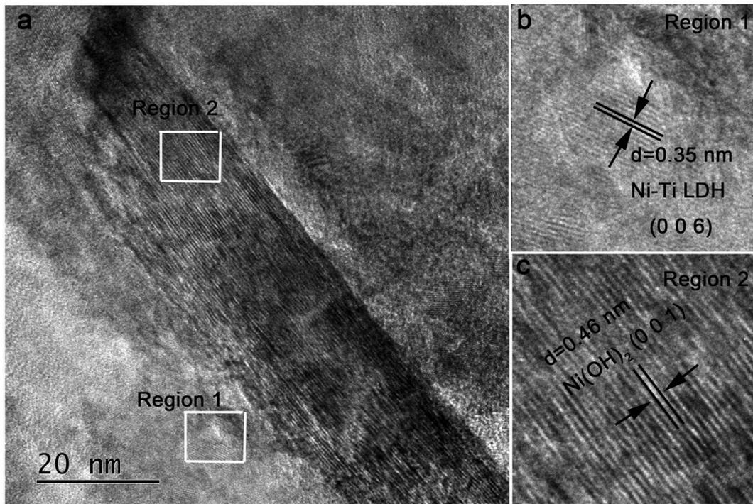
Fig. S1 The HRTEM image of Se0# (a) which show the existence of Ni-Ti LDH (a) and Ni(OH)<sub>2</sub> (c).
