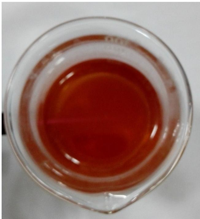
Fig. S5 Photo shows the Tyndall effect of the prepared selenium sol.
