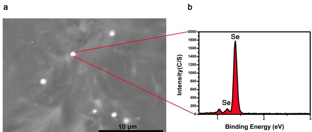
**Fig. S4** SEM images of the prepared nano selenium (a), and the corresponding EDS pattern (b).
