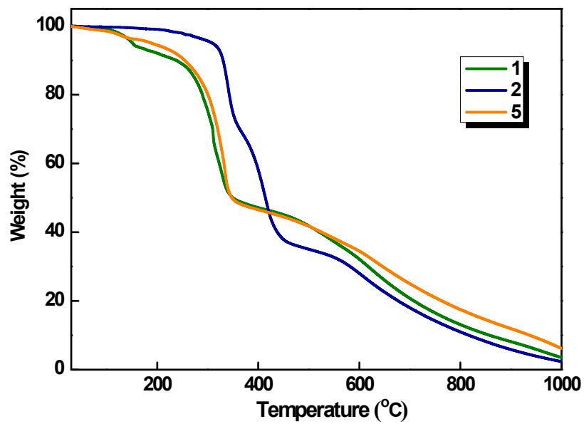
**Fig. S9.** Thermogravimetric curves for complexes **1**, **2** and **5**
