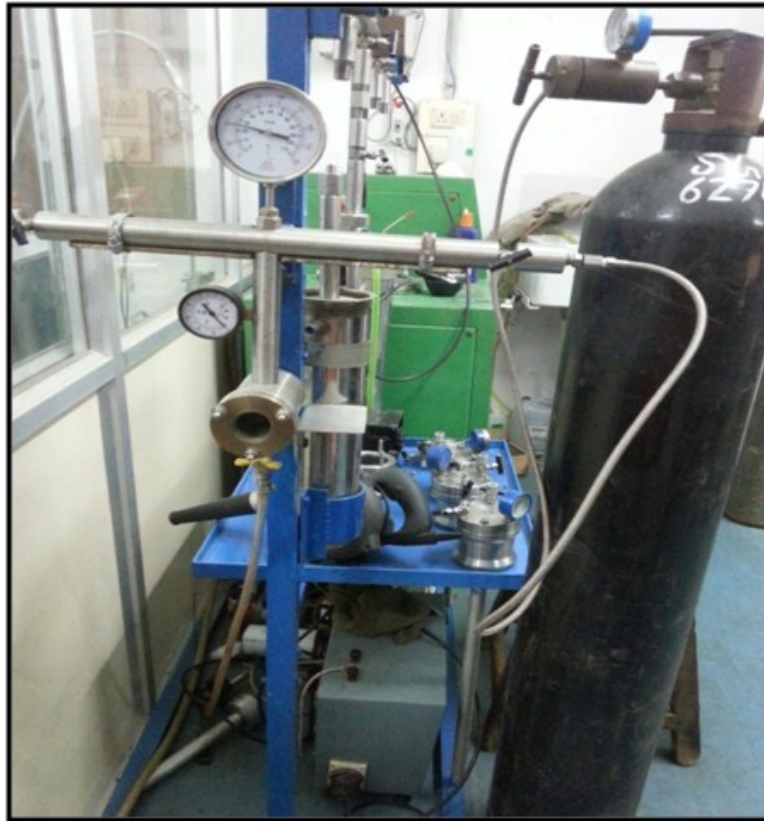
Fig. S4 Locally fabricated Supercritical Dryer.
