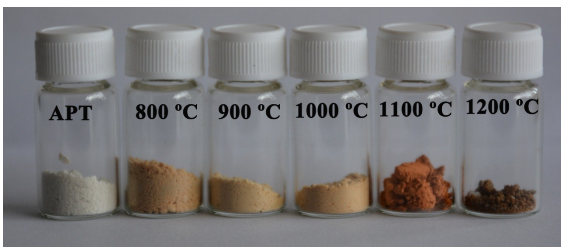
Fig. S2 Digital photographs of the natural APT and the calcined APT at different temperatures.
