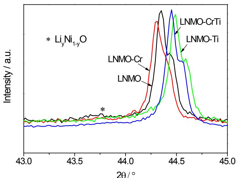
Fig. S1 Magnified image of the XRD pattern between  $43\text{--}45^\circ$
