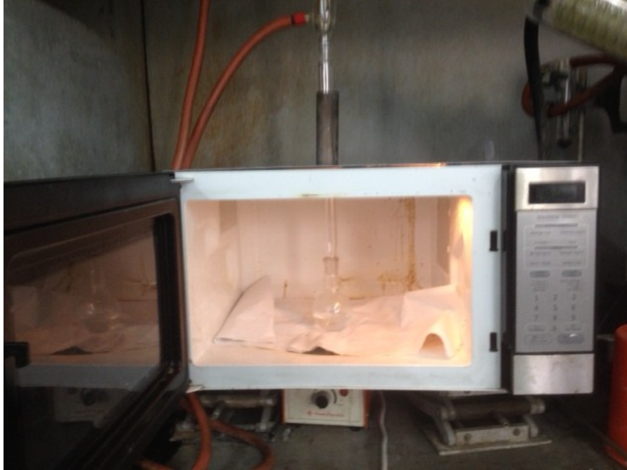
Fig. S2. Digital photograph of the modified domestic microwave oven (MDMWO) with stirring facility used for the hydrolysis of pretreated rice straw
