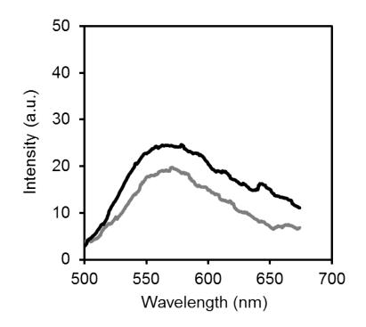
**Figure S1.** Radioluminescence spectra of the film samples of **P6** before (black line) and after (gray line) the X-ray irradiation (60 Gray).
