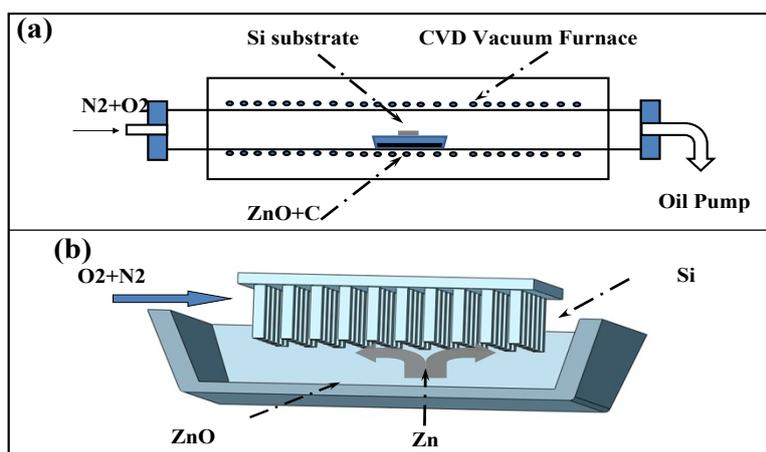
Fig. S3. The process of ZnO nanowire growth by CVD.
