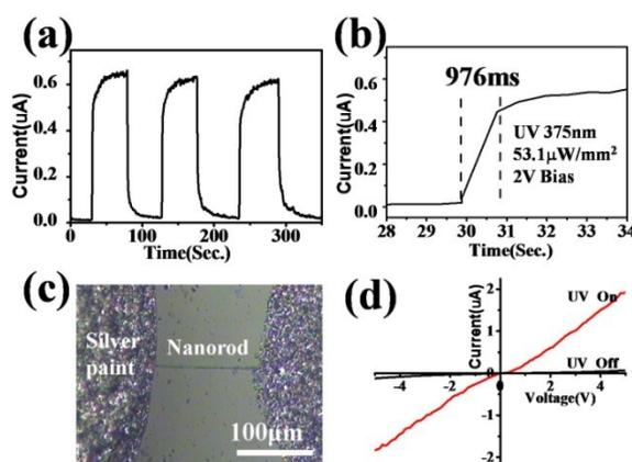
Fig. S1. UV light response results of UV sensor based on single ZnO nanowire. (a) is the on-off ratio; (b) Response time (976 ms); (c) Single ZnO nanowire UV detector; (d) I–V characteristics of the device exposed to 375 nm light with different power densities.
