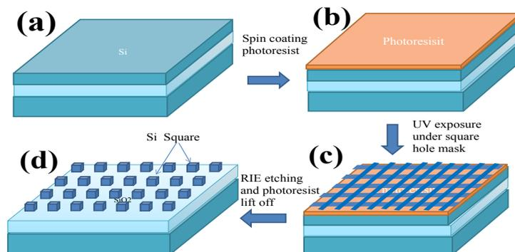
Fig. S2. The fabrication process of SiO<sub>2</sub> nanorod with RIE method.
