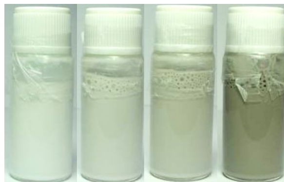
Figure S1. Photographs of 5.0 wt.% PS latex (sample B) with 0.0, 0.05, 0.10, and 0.50 wt.% CuO NP content (from left to right).
