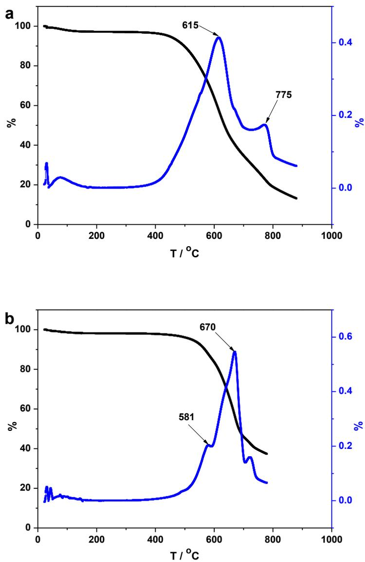
**Figure S3.** TGA of (a) CoPc/g-C<sub>3</sub>N<sub>4</sub>-480 (0.66) and (b) CuPc/g-C<sub>3</sub>N<sub>4</sub>-480 (0.75).
