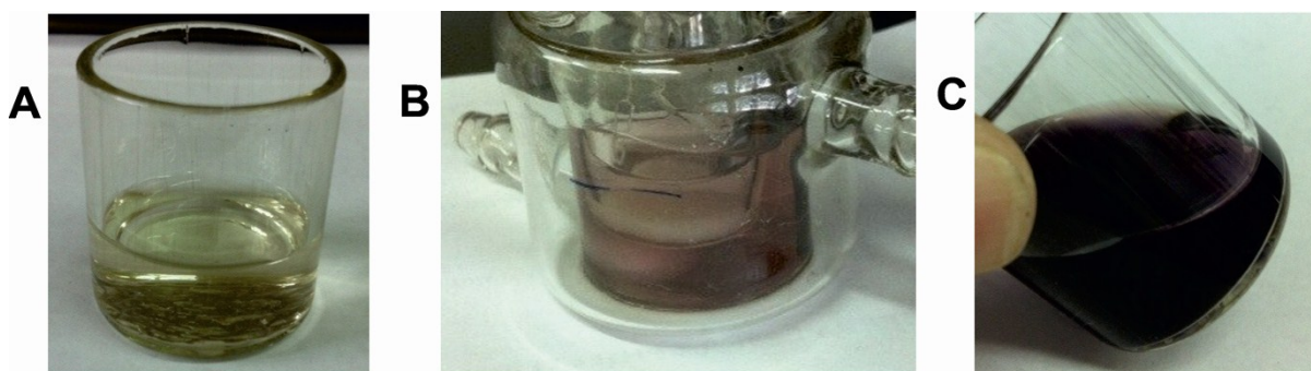
Fig. S5 A picture of 2.0 mM MV^{2+} + 1.5 mM AuCl + 75 mM PVP solutions in H_2O/0.1 M NaCl: starting solution (1) and solution after reduction at -0.90 V at Q = 0.2 F (2) and 1.1 F (3) with respect to AuCl.
