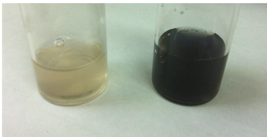
Fig. S2 A picture of 2.0 mM MV 2+ + 1.5 mM AuCl + 1 g/l SiO 2 -NHR solutions in H 2 O/0.1 M NaCl: starting solution (left) and solution after reduction at -0.90 V ( Q = 1.3 F with respect to AuCl) (right).
