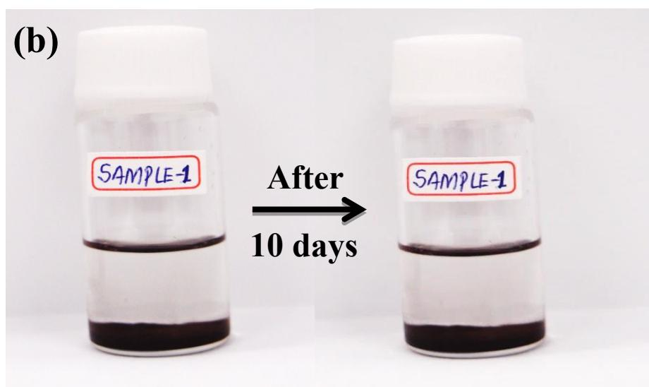
**Fig. S4.** Immersion tests of LNCA powder in (a) 0% IL-incorporated and (b) 75% IL-incorporated electrolytes at 80 °C for 10 days.
