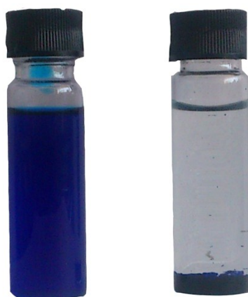
Fig. S8 Photographs of dye solutions before (left) and after (right) adsorption process.
