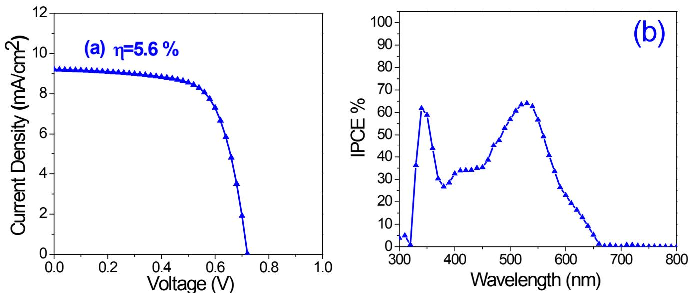
Fig. S3. I–V characteristics of DSSCs made from the pure TiO<sub>2</sub> (a), and IPCE % of pure TiO<sub>2</sub> nanoparticles (b), respectively.
