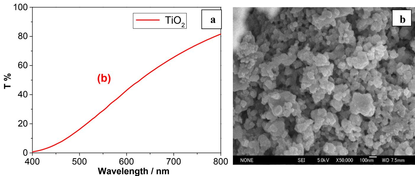
Fig. S1. FESEM patterns of the pure TiO<sub>2</sub> nanoparticles (a), and UV-vis T % of pure TiO<sub>2</sub> nanoparticles (b), respectively.
