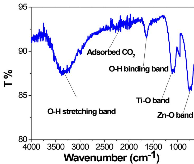
Fig. S2. FTIR T % versus wavenumber (cm<sup>-1</sup>) of ZnO/ TiO<sub>2</sub> nanocomposite.
