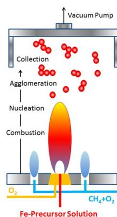
Fig. S1 Schematic of flame spray pyrolysis reactor
