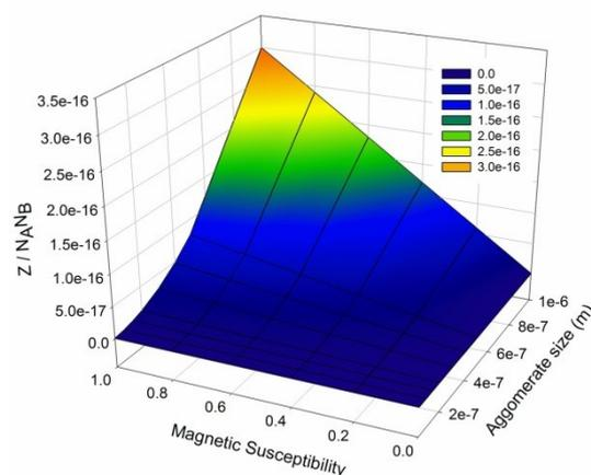
Fig. S4 Plot of collision frequency ratio showing square-dependence on agglomerate size and linear dependence on magnetic susceptibility of the material.
