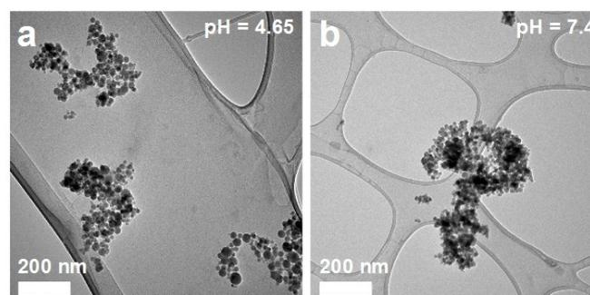
Fig. S3 Transmission Electron Micrographs of FSP-made iron oxide nanoparticles ([Fe]/O<sub>2</sub> = 0.9 mmol/L) encapsulated with lysine at (a) pH 4.65 and (b) 7.4.
