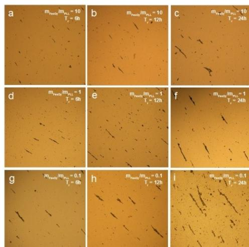
Fig. S2 Optical microscope images showing the effect of reaction time and lysine concentration on morphology of micro-bars synthesized at HAS = 2.5cm, pH 8.8 using FSP-made nanoparticles made at [Fe]/O<sub>2</sub> = 0.9 mmol/L.
