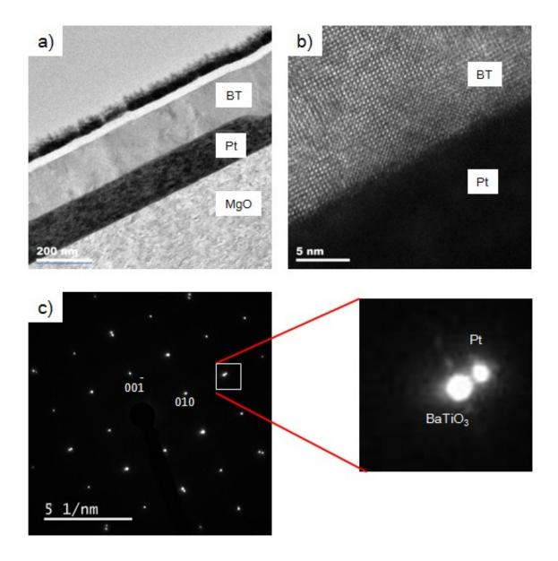
Fig. S2 (a) Cross-sectional TEM images of the  $BaTiO_3(100)$  film on Pt(100)/MgO(100), (b) boundary of the  $BaTiO_3(100)$  film and Pt(100) film, and (c) SAED of boundary of the  $BaTiO_3(100)$  film and Pt(100) film.
