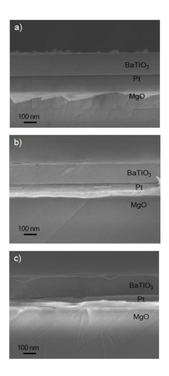
Fig. S1 Cross-sectional FE-SEM image of (a)  $BaTiO_3(100)$  film on a Pt(100)/MgO(100) substrate, (b)  $BaTiO_3(110)$  film on a Pt(110)/MgO(110) substrate, and (c)  $BaTiO_3(111)$  on a Pt(111)/MgO(111) substrate.
