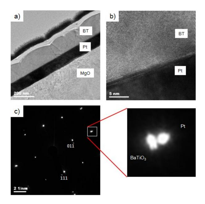
Fig. S4 (a) Cross-sectional TEM images of the  $BaTiO_3(111)$  film on Pt(111)/MgO(111), (b) boundary of the  $BaTiO_3(111)$  film and Pt(111) film, and (c) SAED of boundary of the  $BaTiO_3(111)$  film and Pt(110) film.
