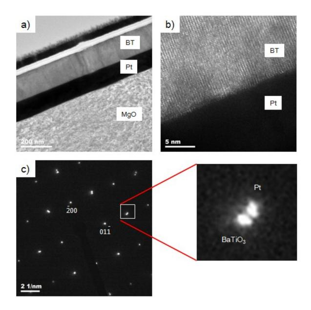
Fig. S3 (a) Cross-sectional TEM images of the  $BaTiO_3(110)$  film on Pt(110)/MgO(110), (b) boundary of the  $BaTiO_3(110)$  film and Pt(110) film, and (c) SAED of boundary of the  $BaTiO_3(110)$  film and Pt(110) film.
