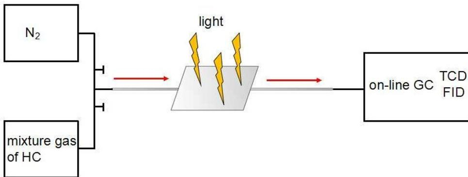
Figure S2 The schematic diagram of continues flow photocatalytic test
