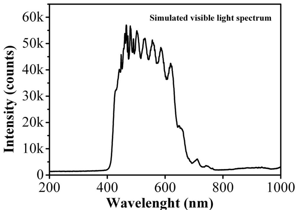
**Figure S4** The visible light spectrum of simulated solar light
