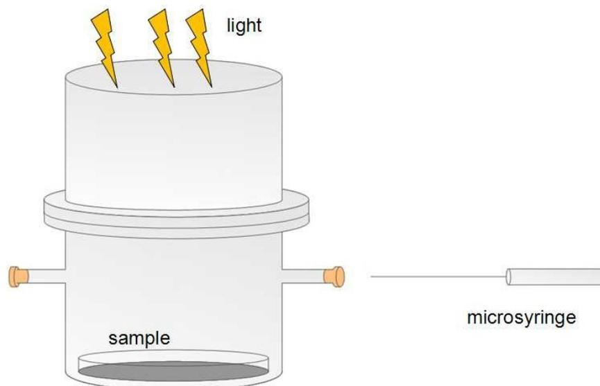
**Figure S1** The sketch of photoreaction in a sealed quartz reactor
