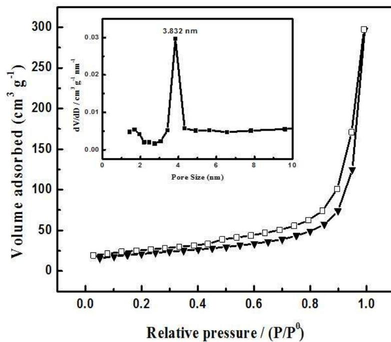
Fig.S1 N<sub>2</sub> adsorption-desorption isotherm at 77k of the as-formed “desert rose”-like structure MnO<sub>2</sub> and the inset shows the corresponding pore size distribution calculated by the BJH method from the desorption branch of the isotherm.
